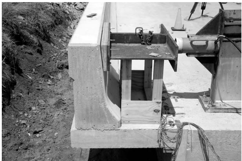
Figure 6. Test Setup for Static Load Testing.
