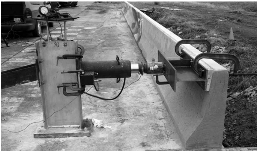
Figure 18. Test Setup for Static Load Testing.
