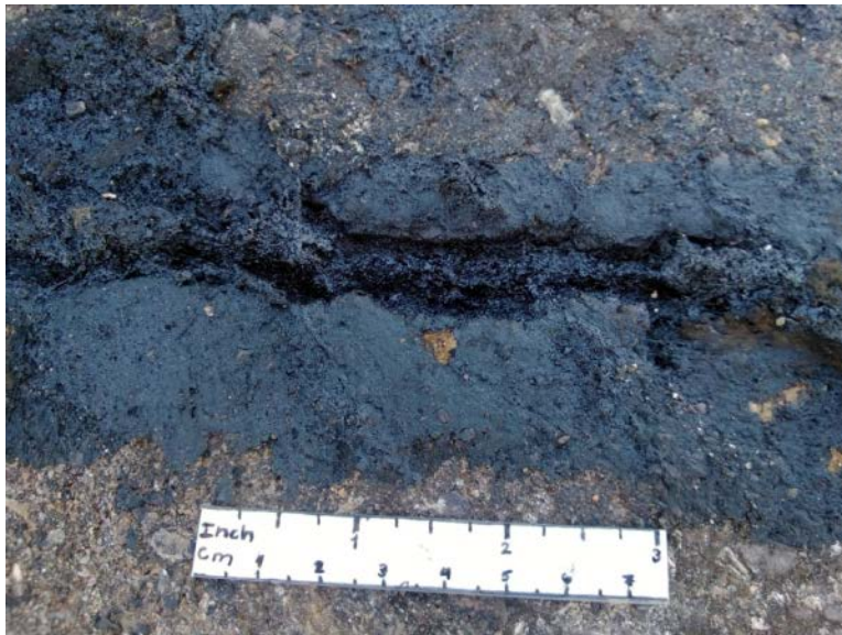
Figure 11. Polyflex Type II with Routing after Severe Heavy Traffic Test.
