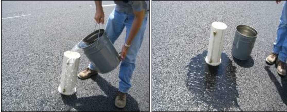
Figure 18. Test Method Tex-246-F, Field Water Flow Test.
