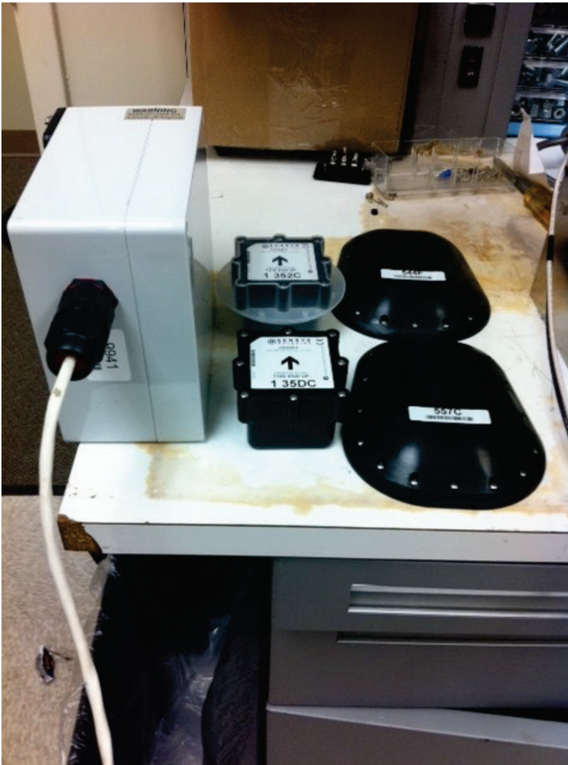
Figure 12. Four Sensys Sensors and an Access Point Necessary to Operate the Beacon.
