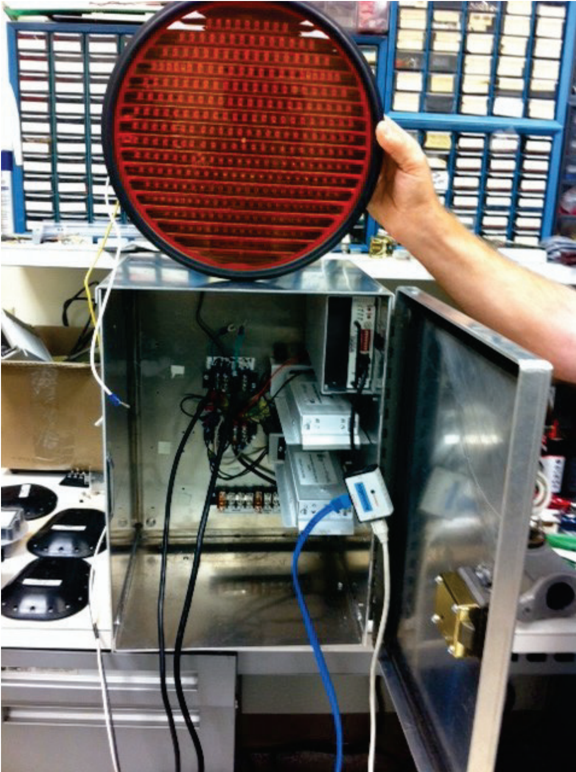
Figure 11. A Fabricated Flasher Panel to Control the Beacons Using Sensys Sensors.
