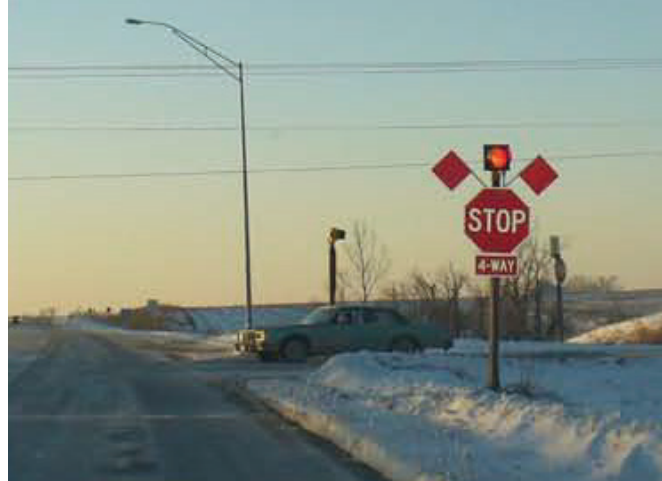
Figure 8. Examples of Replacement Beacons for Overhead Flashing Beacons.
