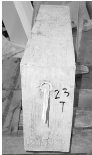
Figure 78. Bar Rupture Failure.
