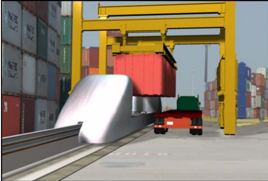
Figure 17. Transfer of Freight Shuttle Cargo Using Container Cranes.
