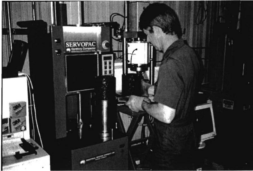
Figure B1. Superpave Gyrotory Compactor.
