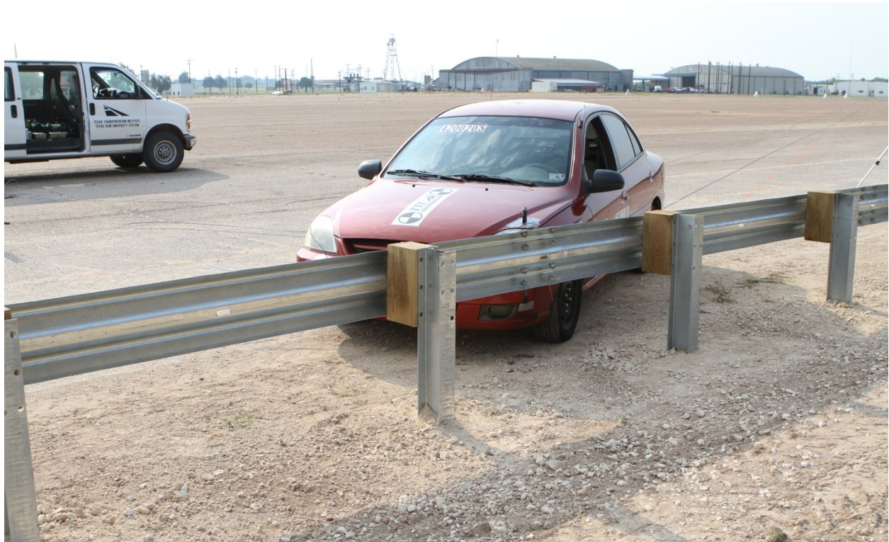
Figure 5.1. Vehicle/Installation Geometrics for Test No. 420020-5.
