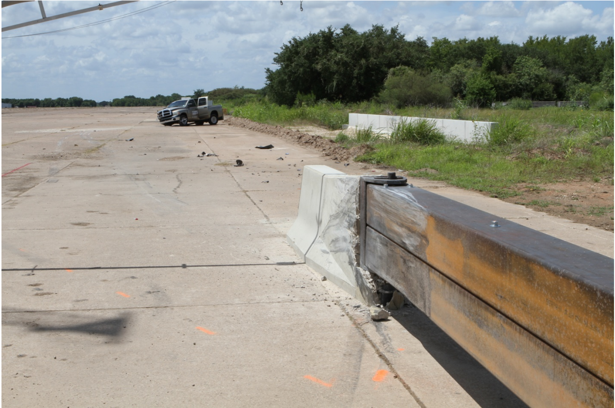
Figure 8.3. Position of Vehicle/Gate after Test No. 420020-8.
