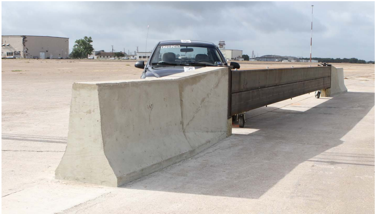
Figure 6.1. Vehicle/Barrier Geometries for Test No. 420020-6.
