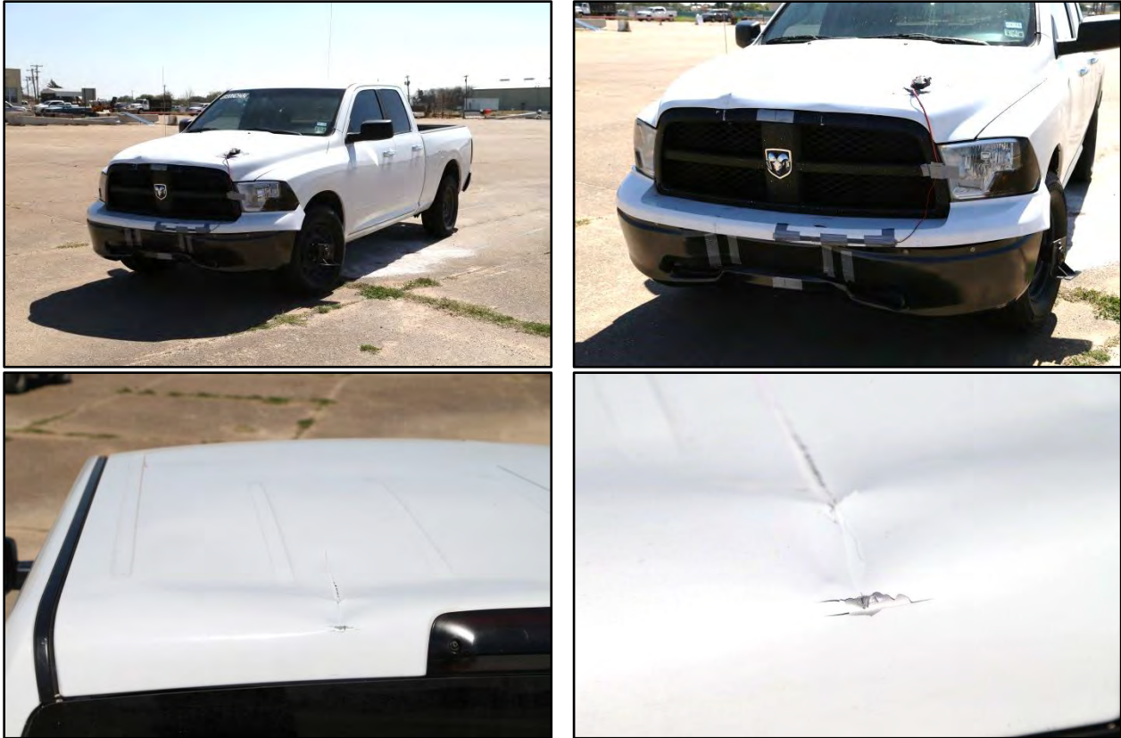
Figure 6.5. Test Vehicle after Test No. 490026-2-2.
