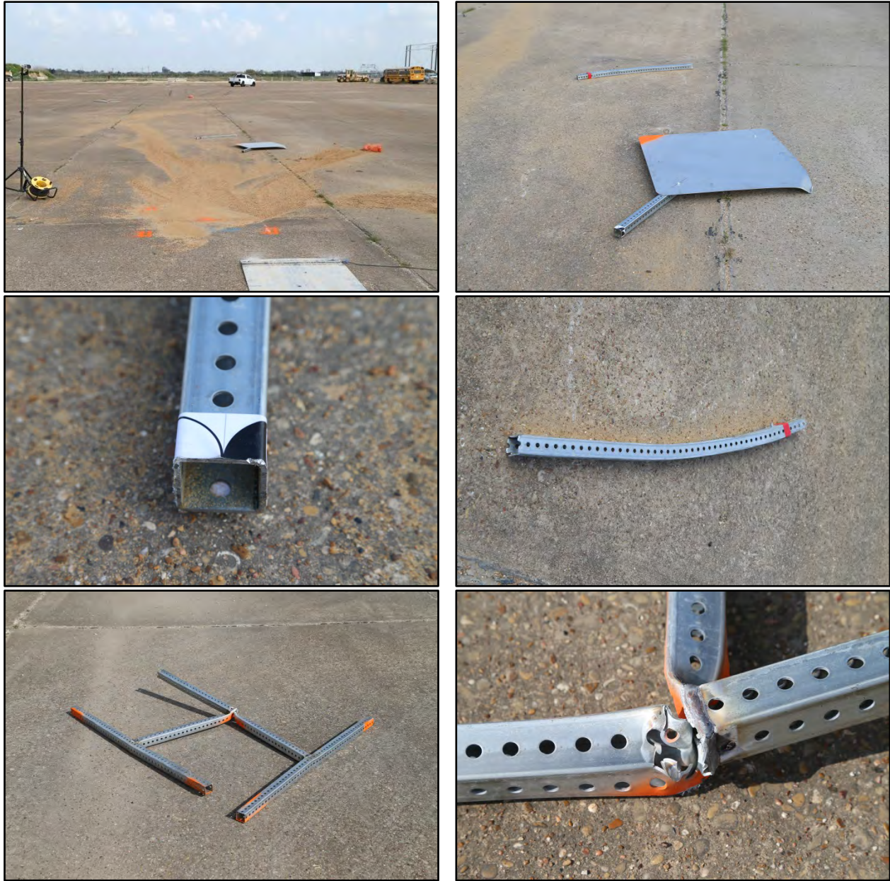
Figure 5.4. Option A Temporary Work Zone Sign Support after Test No. 490026-2-1.
