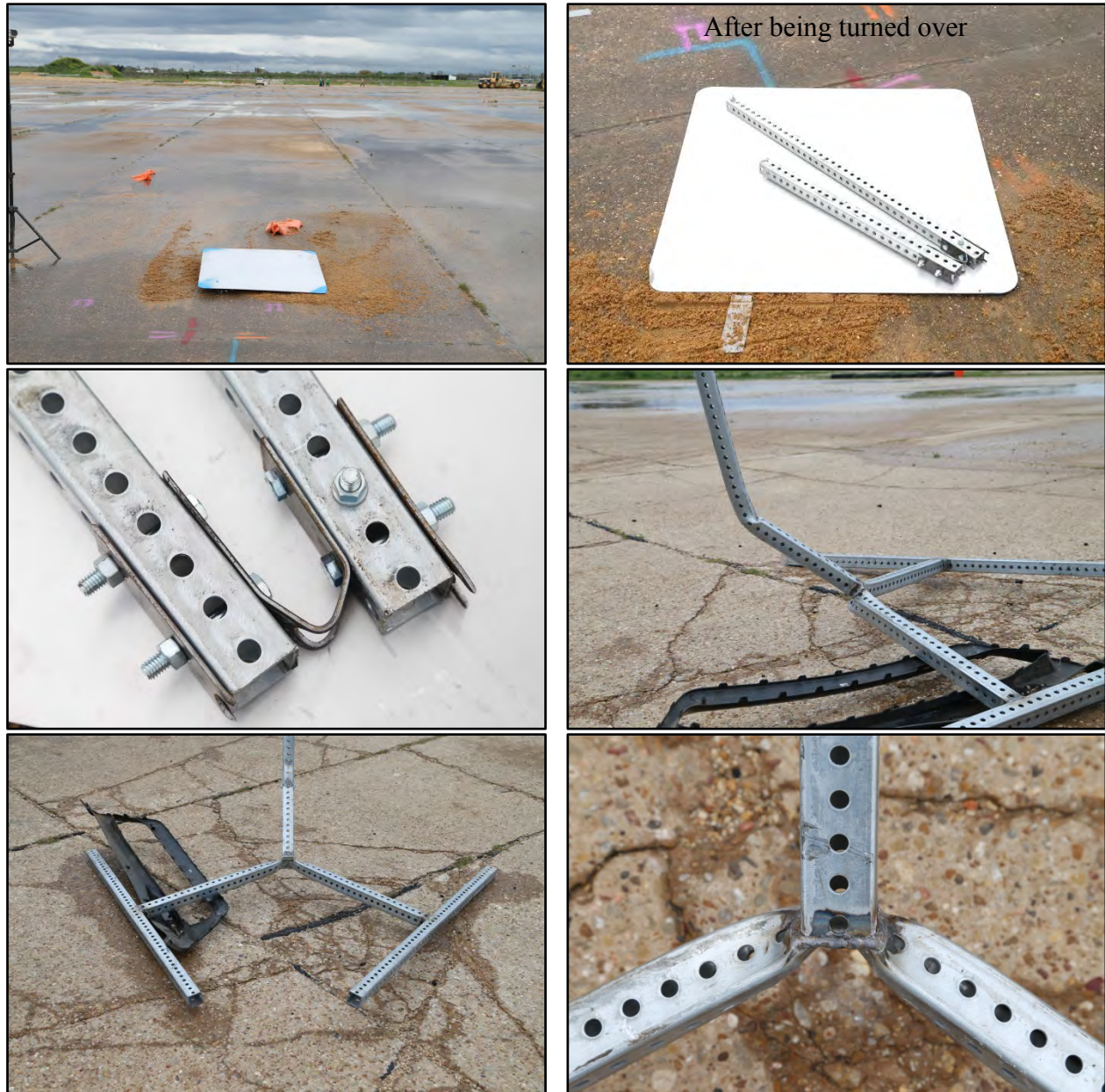
Figure 6.10. Option B Temporary Work Zone Sign Support after Test No. 490026-2-4.
