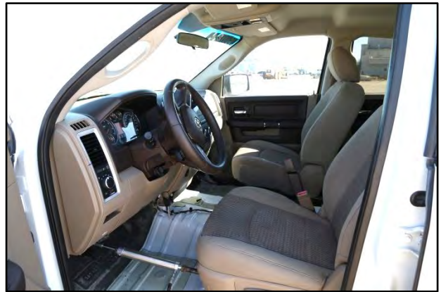
Figure 6.24. Interior of Test Vehicle after Test No. 490026-2-8.
