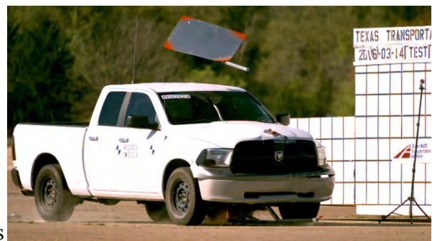
Figure E.1. Sequential Photographs for Test No. 490026-2-8 (Perpendicular and Oblique Views).
