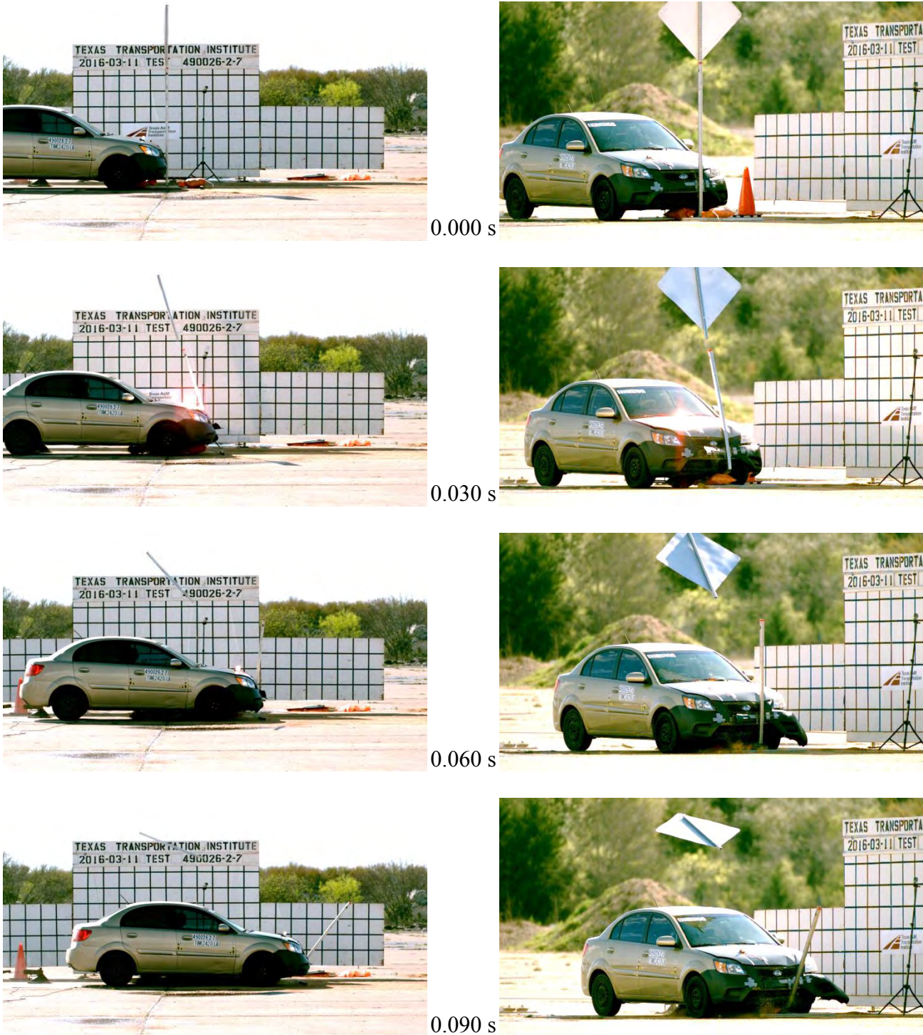
Figure H.1. Sequential Photographs for Test No. 490026-2-7 (Perpendicular and Oblique Views).
