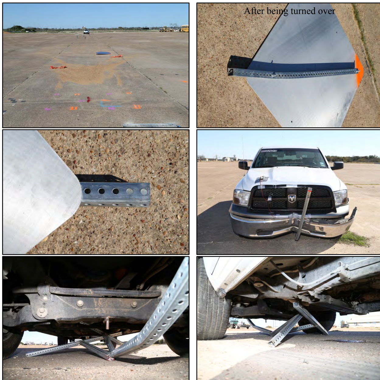
Figure 7.4. Option C Temporary Work Zone Sign Support after Test No. 490026-2-3.
