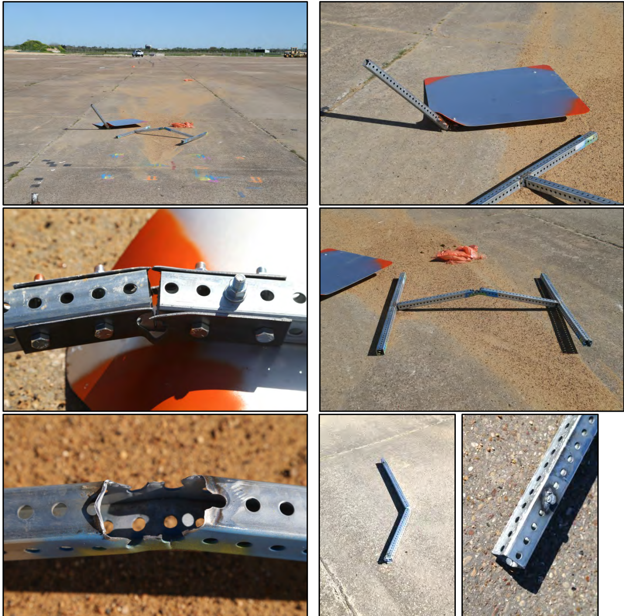
Figure 6.22. Option A Temporary Work Zone Sign Support after Test No. 490026-2-8.
