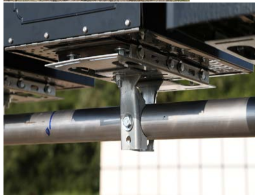
Figure 5.4. Locking Architectural and Standard Mailboxes on 11-Gauge Steel Tube Multiple Mailbox Support before Testing.
