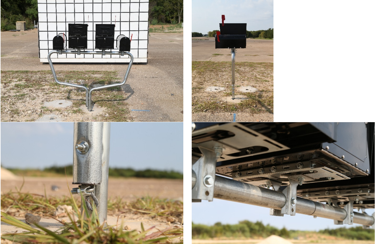
Figure 6.4. Locking Architectural and Standard Mailboxes on 16-Gauge Steel Tube Multiple-Mailbox Support before Testing.
