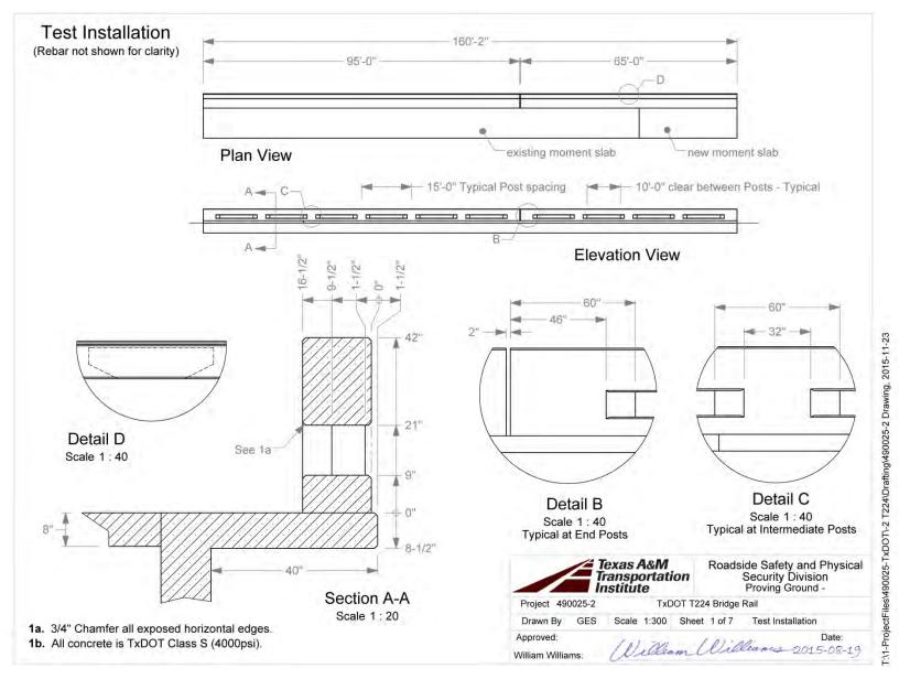
Figure 2.1. Overall Details of the TxDOT T224 Bridge Rail.
