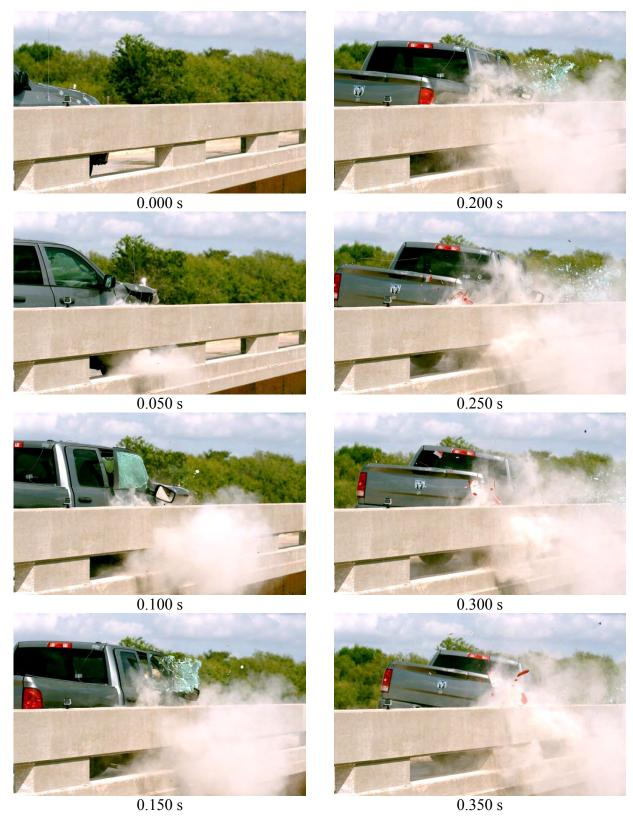
Figure D.2. Sequential Photographs for Test No. 490025-2-3 (Rear View).
