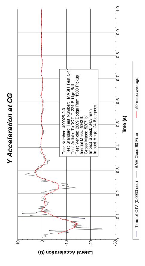
Figure D.5. Vehicle Lateral Accelerometer Trace for Test No. 490025-2-3 (Accelerometer Located at Center of Gravity).
