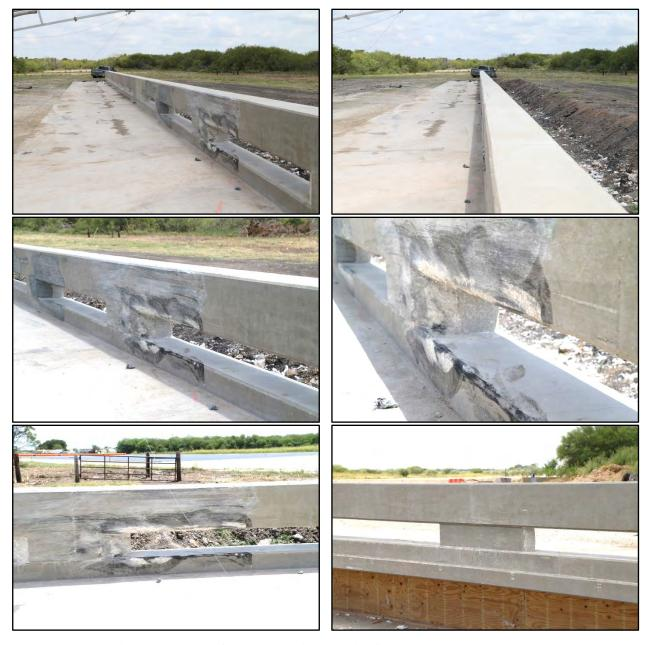
Figure 6.3. TxDOT T224 Bridge Rail after Test No. 490025-2-3.
