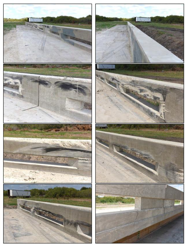
Figure 7.3. TxDOT T224 Bridge Rail after Test No. 490025-2-1.
