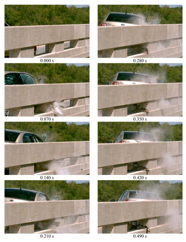
Figure C.2. Sequential Photographs for Test No. 490025-2-2 (Rear View).
