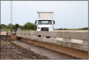
Figure 7.1. TxDOT T224 Bridge Rail/Test Vehicle Geometrics for Test No. 490025-2-1.
