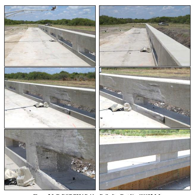
Figure 5.3. TxDOT T224 Bridge Rail after Test No. 490025-2-2.
