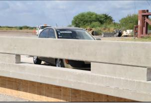
Figure 5.1. TxDOT T224 Bridge Rail/1100C Vehicle Geometrics for Test No. 490025-2-2.
