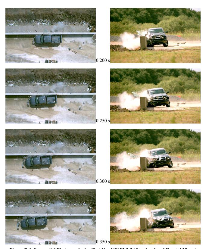
Figure D.1. Sequential Photographs for Test No. 490025-2-3 (Overhead and Frontal Views) (Continued).
