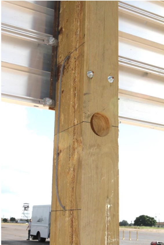
Figure 2.2. Temporary Wood Sign Support for Large Guide Signs before Testing.
