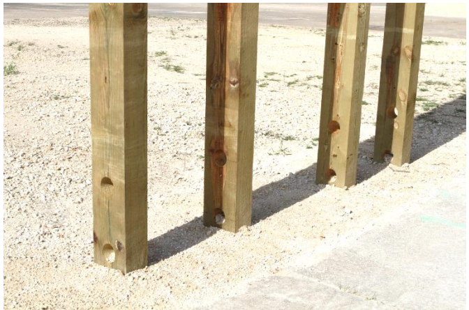
Figure 2.2. Temporary Wood Sign Support for Large Guide Signs before Testing.
