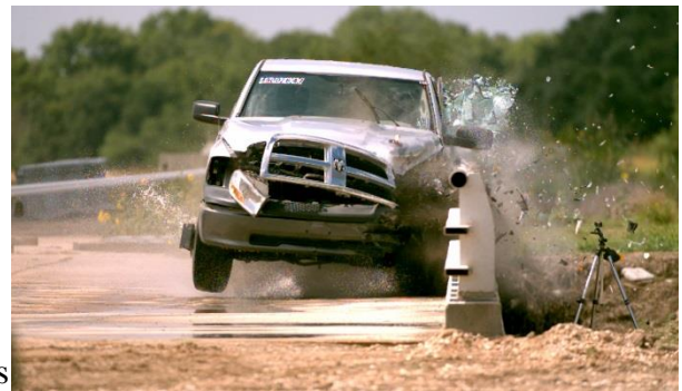
Figure E-1. Sequential Photographs for Test No. 490026-4-2 (Overhead and Frontal Views).
