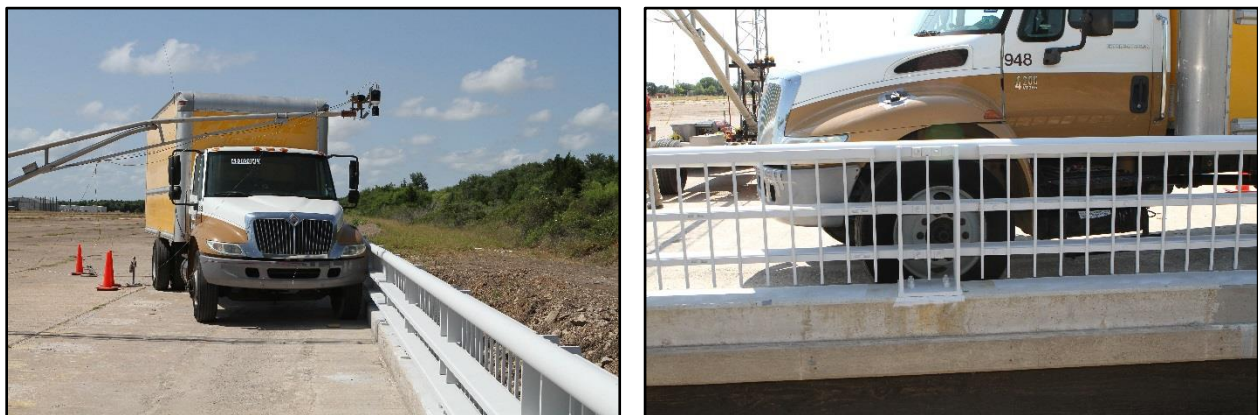
Figure 7-1. TxDOT Type C2P Bridge Rail/Test Vehicle Geometrics for Test No. 490026-4-3.
