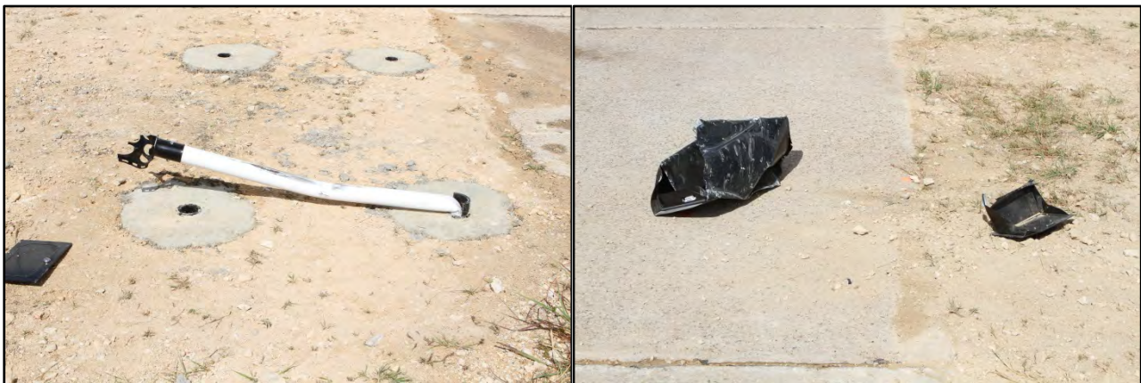
Figure 4.7. Installation after Test No. 490023-9-1.
