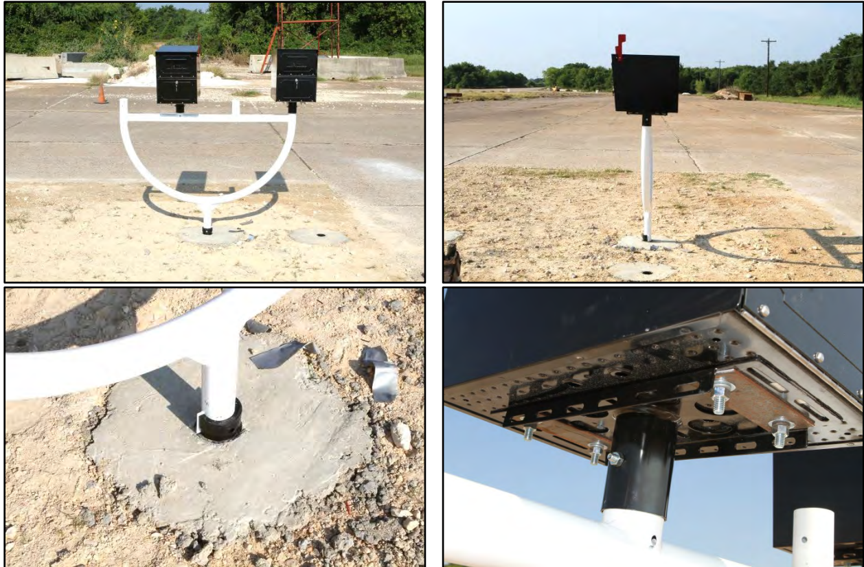
Figure 5.3. Dual Locking Architectural Mailboxes on SHUR-TITE ® Multiple-Mount Post before Testing.
