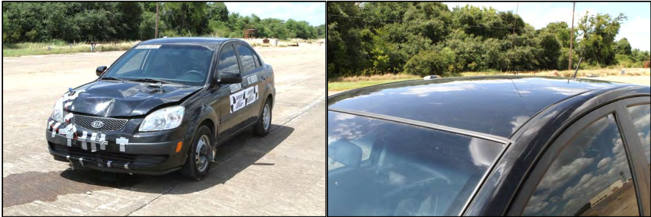
Figure 4.15. Vehicle after Test No. 490023-9-2.
