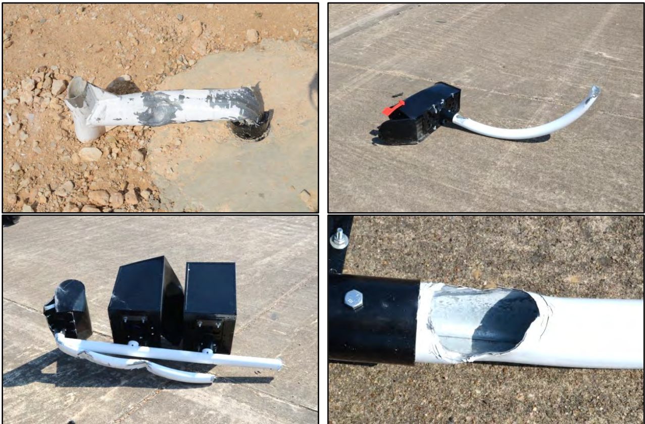
Figure 6.8. Installation after Test No. 490023-9-5.
