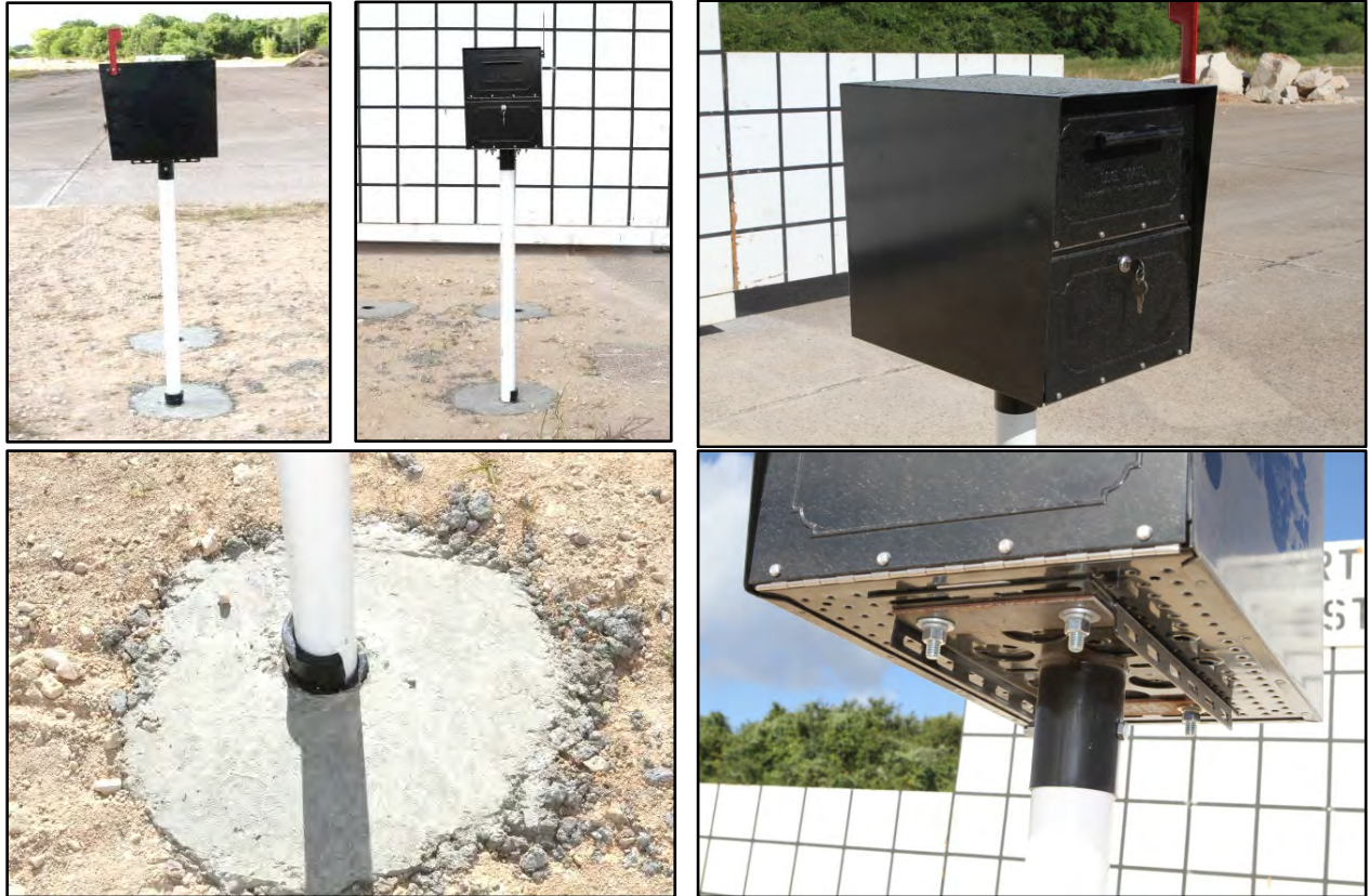
Figure 4.3. Locking Architectural Mailbox on the SHUR-TITE® Single Mount Post before Testing.
