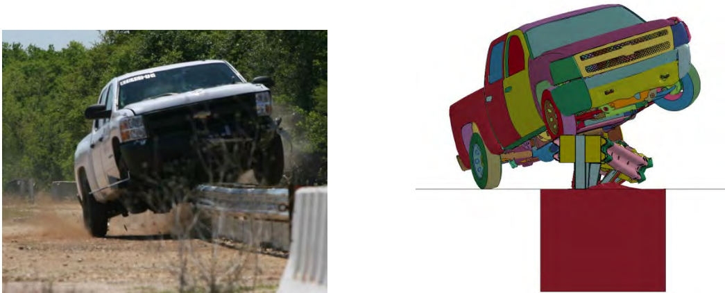
Figure 2.3. Simulation of the MASH 3-11 as the 2270P Vehicle Vaults over the 27-Inch Median Barrier.
