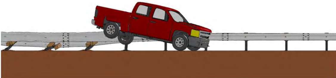
Figure 2.16. Silverado Model at Maximum Pitch for At-Post Impact.
