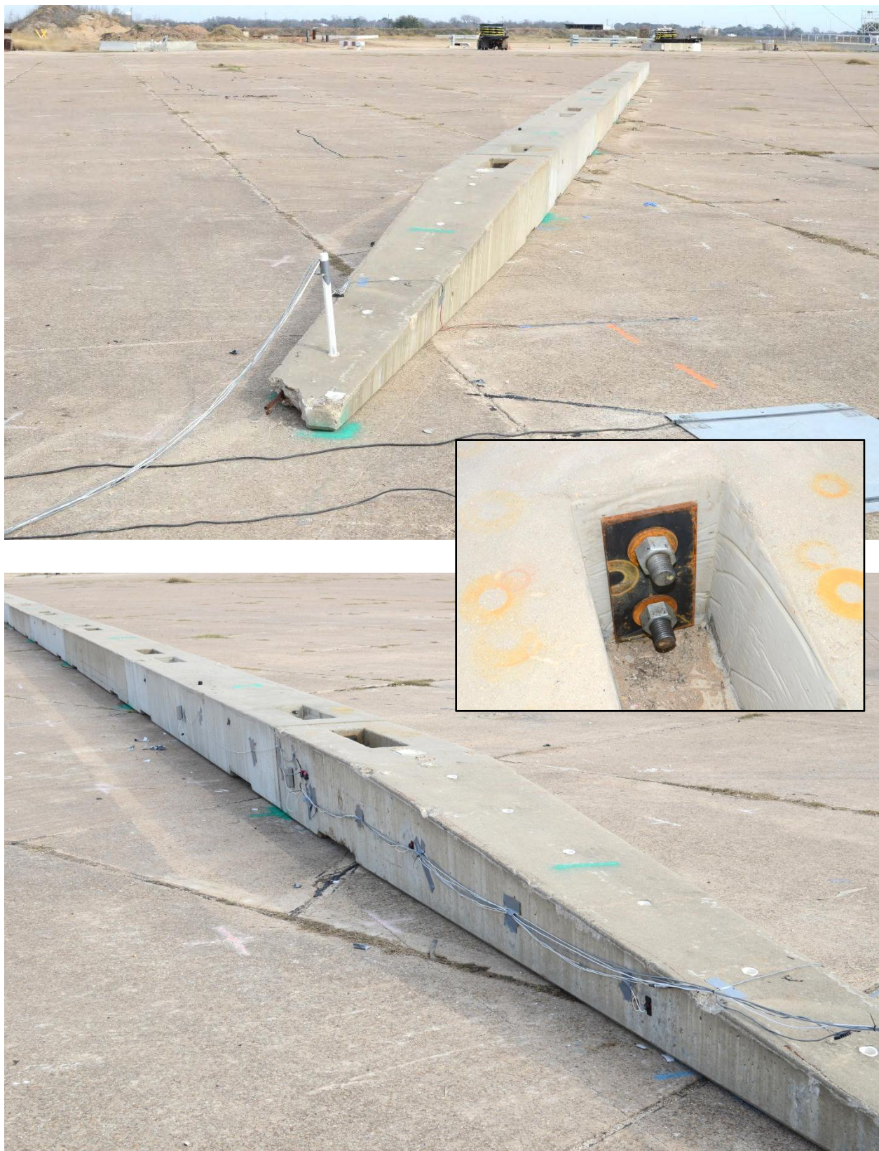
Figure 2.3. Non-pinned Low-Profile End Treatment before Test No. 490023-7.
