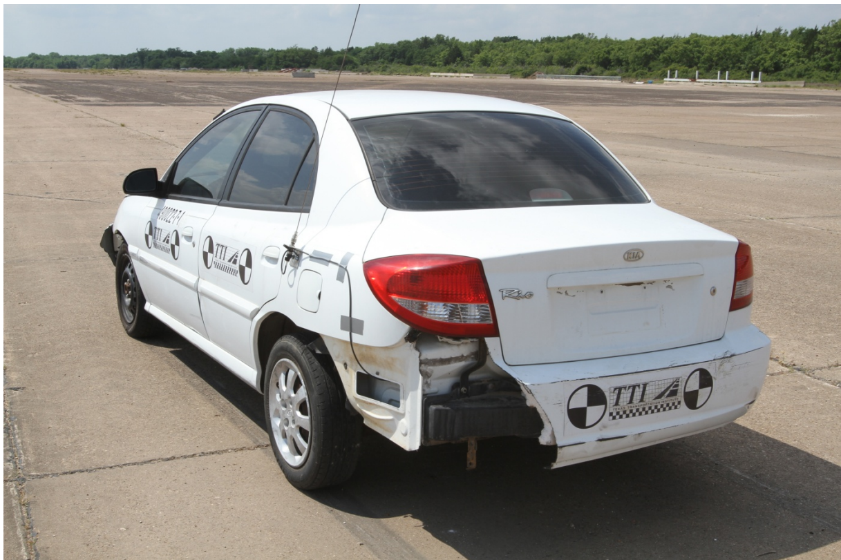
Figure 4.9. Vehicle after Test No. 490022-7-1.
