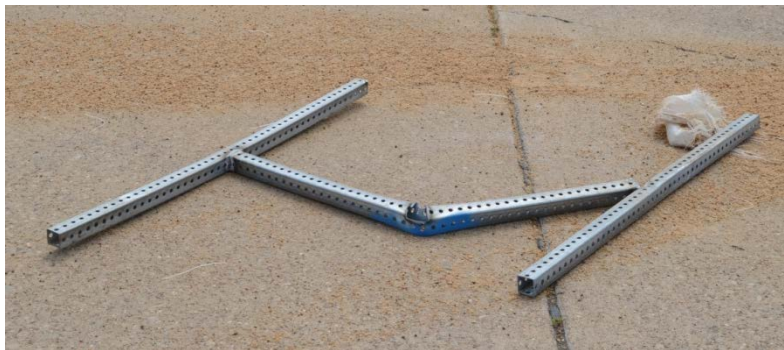
Figure 6.7. Installation after Test No. 490022-7-4.
