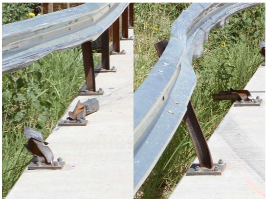
Figure 5.4. Installation after Test No. 490023-6-1a.
