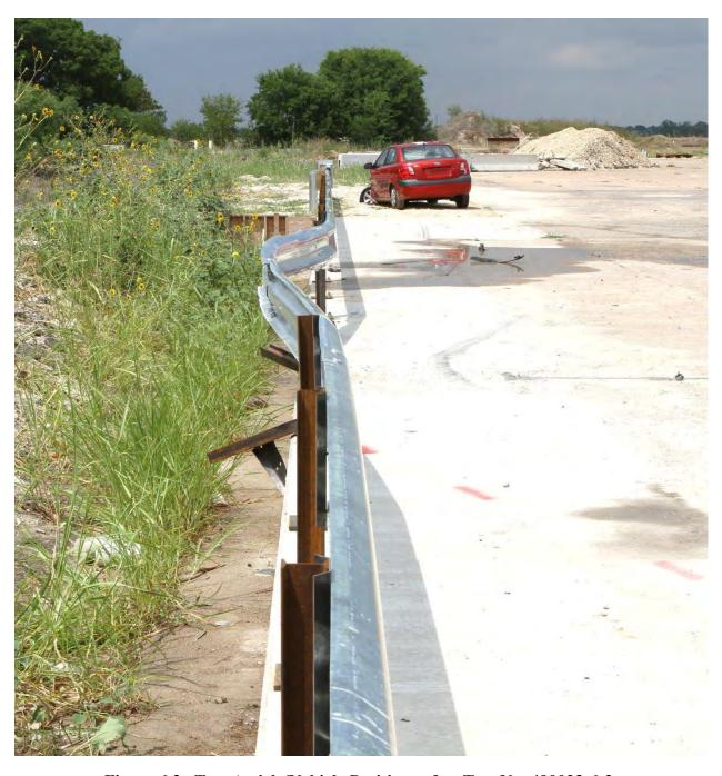
Figure 6.3. Test Article/Vehicle Positions after Test No. 490023-6-2.
