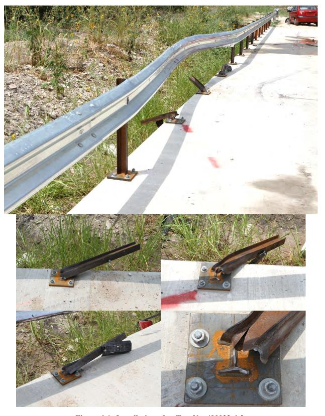
Figure 6.4. Installation after Test No. 490023-6-2.
