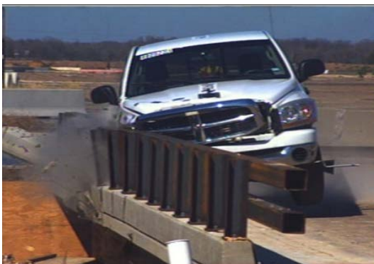
Figure D1. Sequential Photographs for Test No. 490022-1 (Field Side of Bridge Rail).
