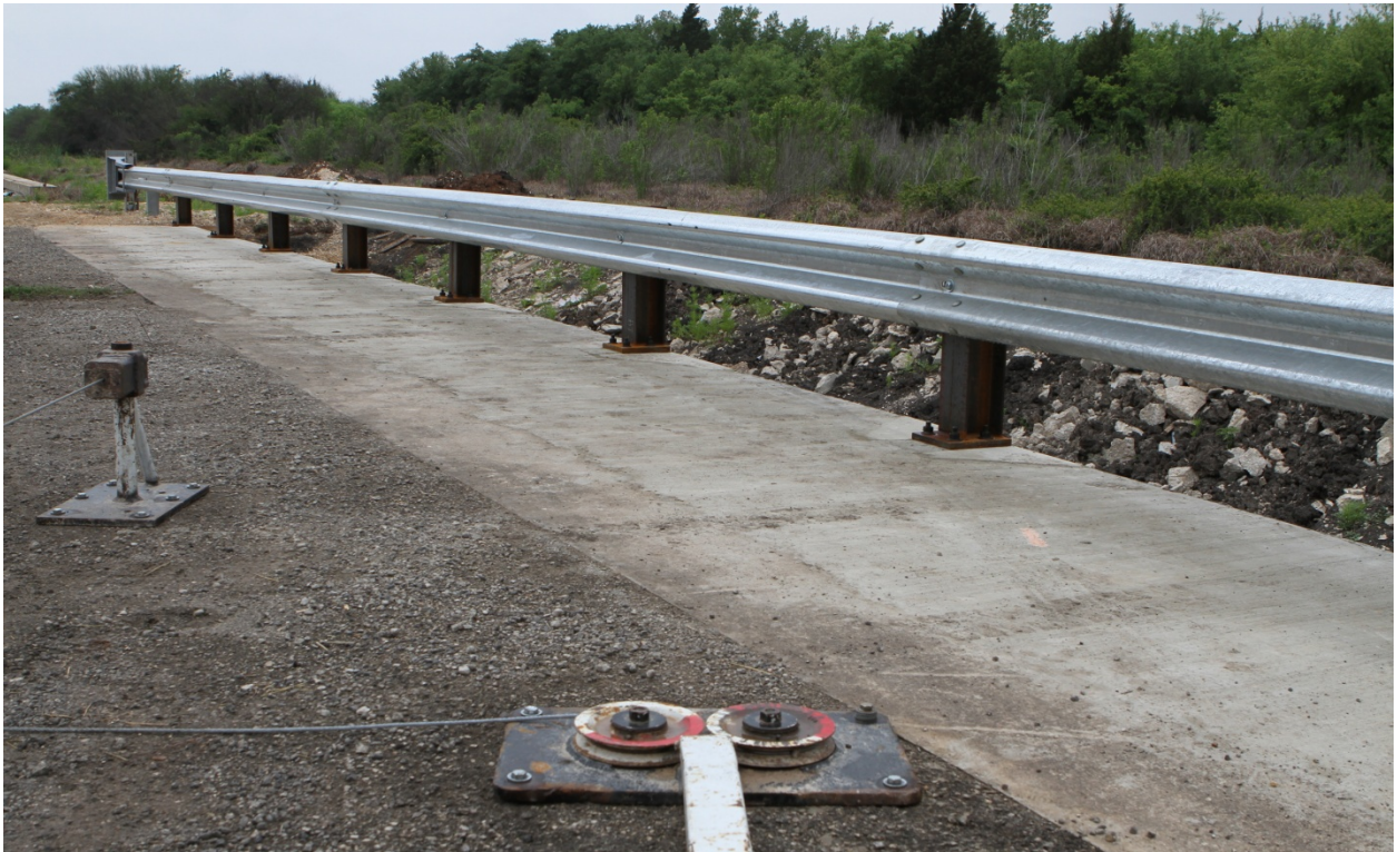
Figure 2.3. T101 Bridge Rail before Test No. 420020-1a.
