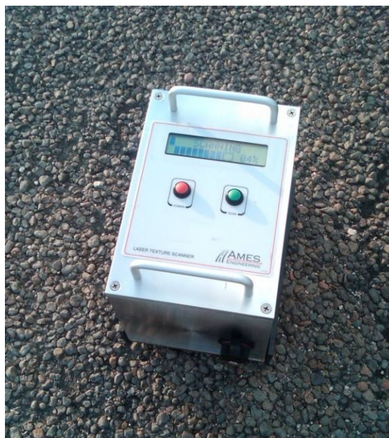
Figure 12. Laser Texture Scanner Taking a Reading.
