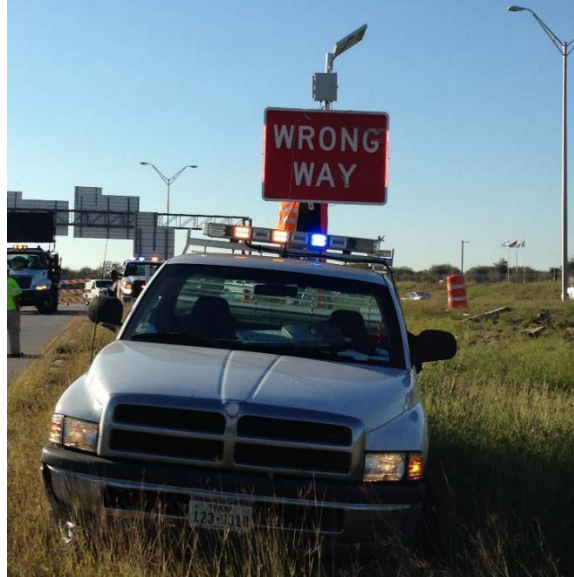
Figure 3. Example of Multiple-Radar Detection WWD Warning System with Flashing LED Panels.
