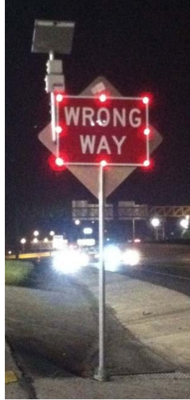
Figure 2. Example of WRONG WAY Sign with Flashing Red LEDs around Border.
