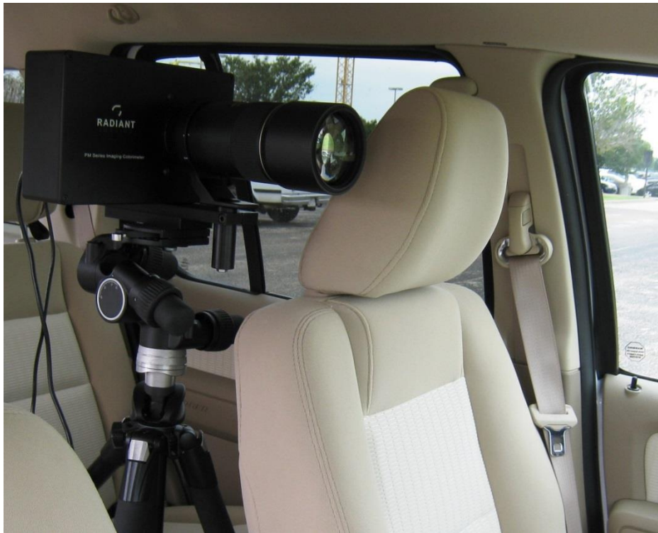
Figure 5. Photometric Camera Installed in Research Vehicle.
