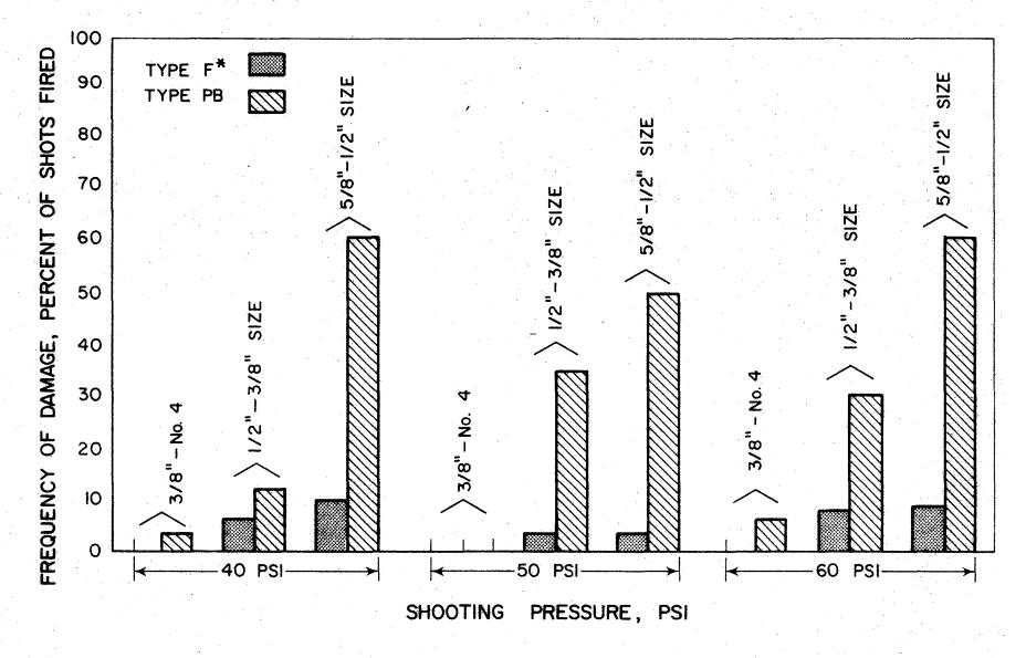
Figure 3. Comparative damage to windshields for Type F\* aggregate and Type PB aggregate shot at different pressures.
