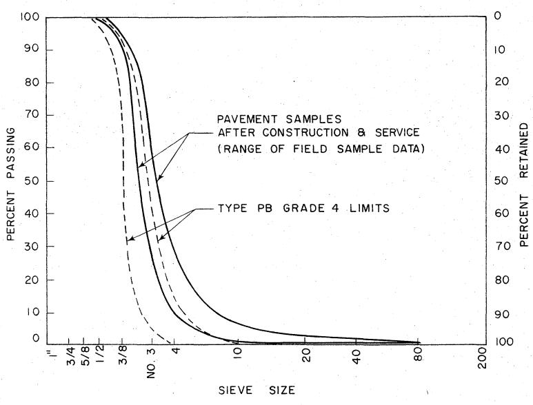
Figure 8. Comparative degradation of precoated limestone due to construction and service (after Gallaway (7)).
