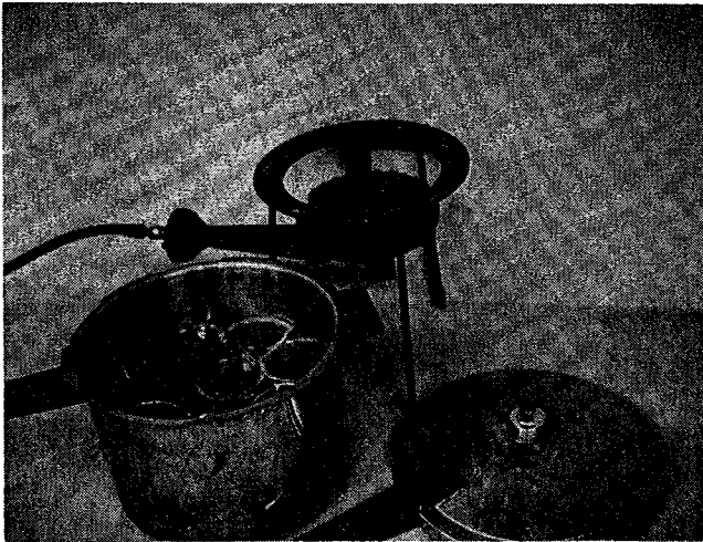
Figure 4. In a later modification to the evaluation test, kiln produced aggregates—after cooking (upper)—are subjected to severe agitation in water by a laboratory heavy duty shaker (lower). This is referred to as the "pressure slaking test."
