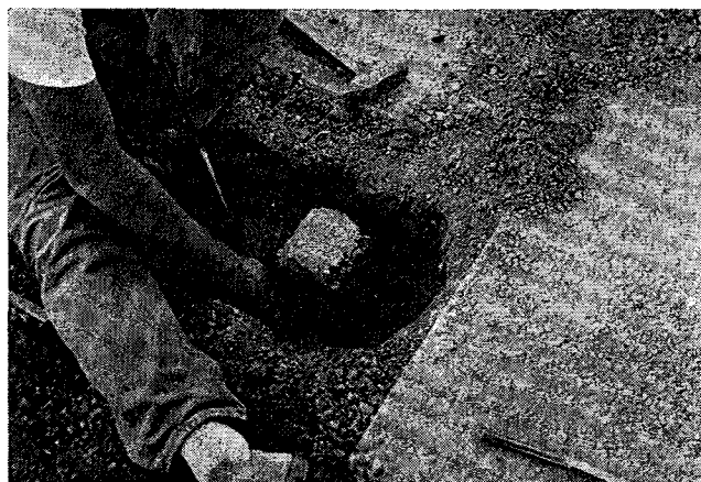
Figure 7. Synthetic flexible bases that had been in service for several years in the Houston area were sampled for laboratory testing.
