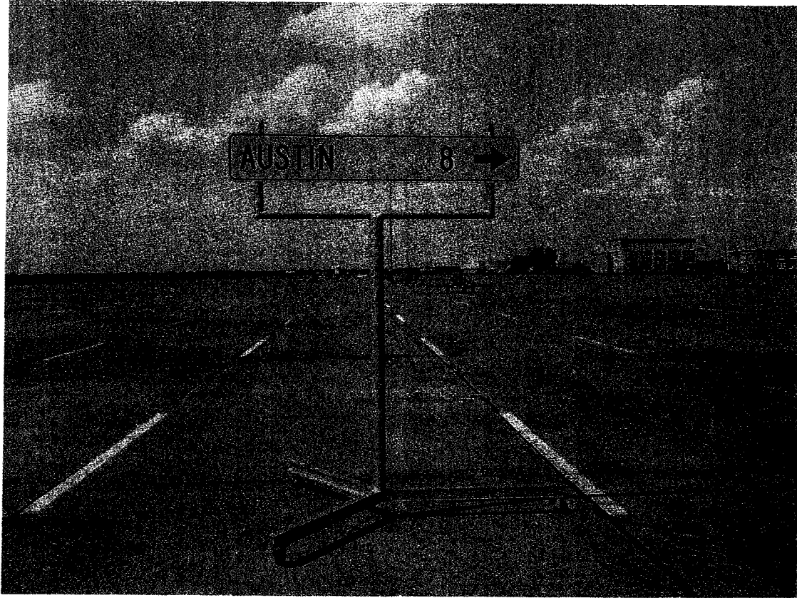
Figure 12. Portable sign frame and test sign.
