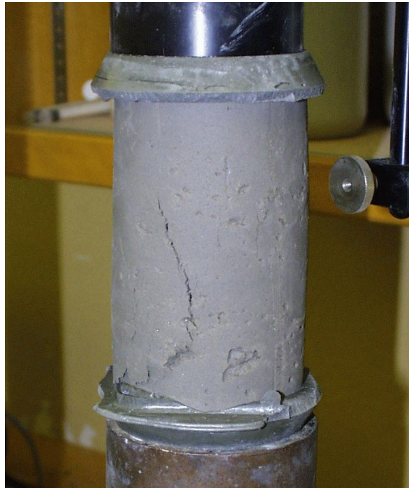
Figure 5.12. Flowable Fill Specimen Failed in Compression.
