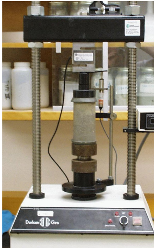
Figure 5.11. Compressive Strength Tests on Flowable Fill Mixtures.
