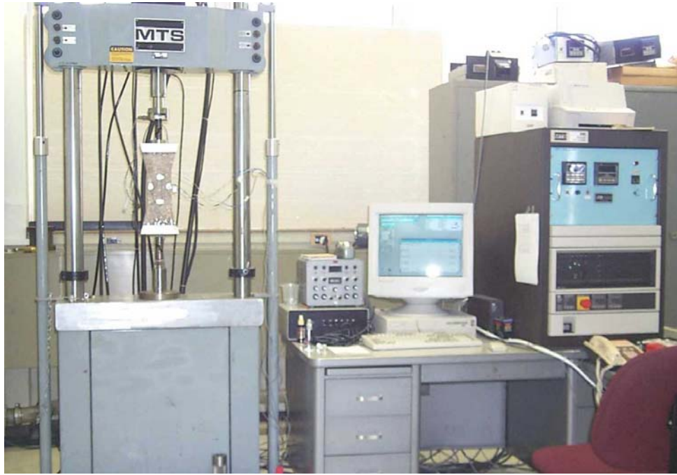
Figure 4.21. Tensile Relaxation Test System.
