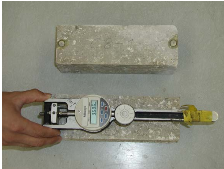
Figure 4.15. Set-Up for Drying Shrinkage Measurement.
