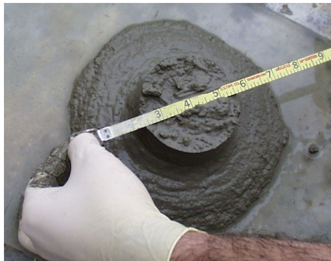
Figure 5.3. Collapsed Flow Specimen and Method Used to Measure Flow.
