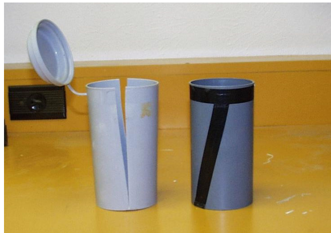
Figure 5.2. Cylinders Used for Flowable Fill Test Specimens. (Shown on the left is a vertically cut cylinder; on the right is a cylinder taped and ready to be filled with fresh flowable fill.)
