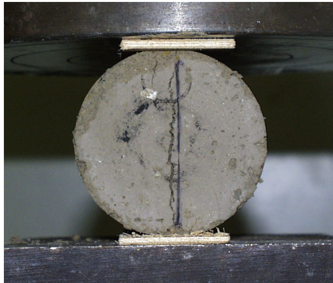
Figure 5.7. Flowable Fill Specimen Failed in Splitting Tension.
