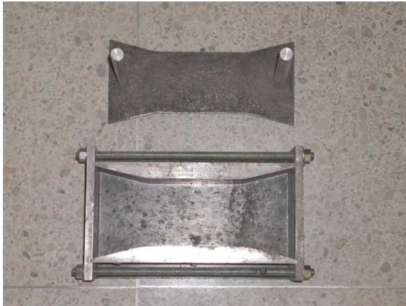
Figure 4.19. Compaction Mold for Relaxation Test Specimen.
