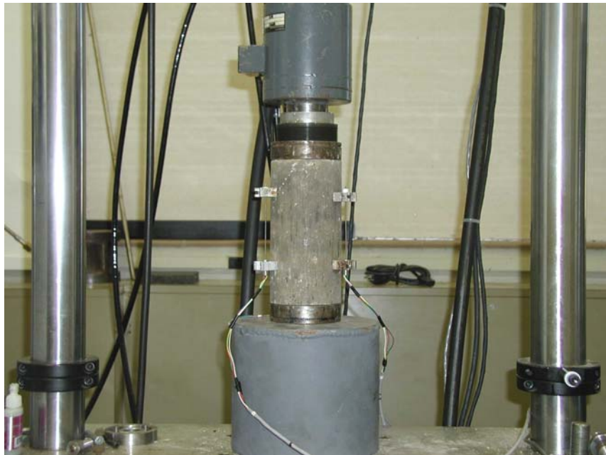
Figure 4.7. Configuration for Uniaxial Compression Tests.
