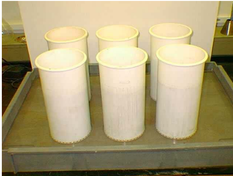
Figure 2. TST Arrangement for Unstabilized Aggregates.
