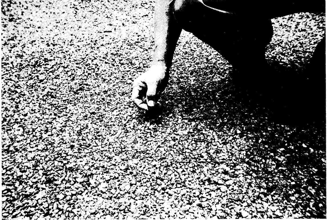
Figure 58. Adhesion of asphalt to Type F material is very good.
