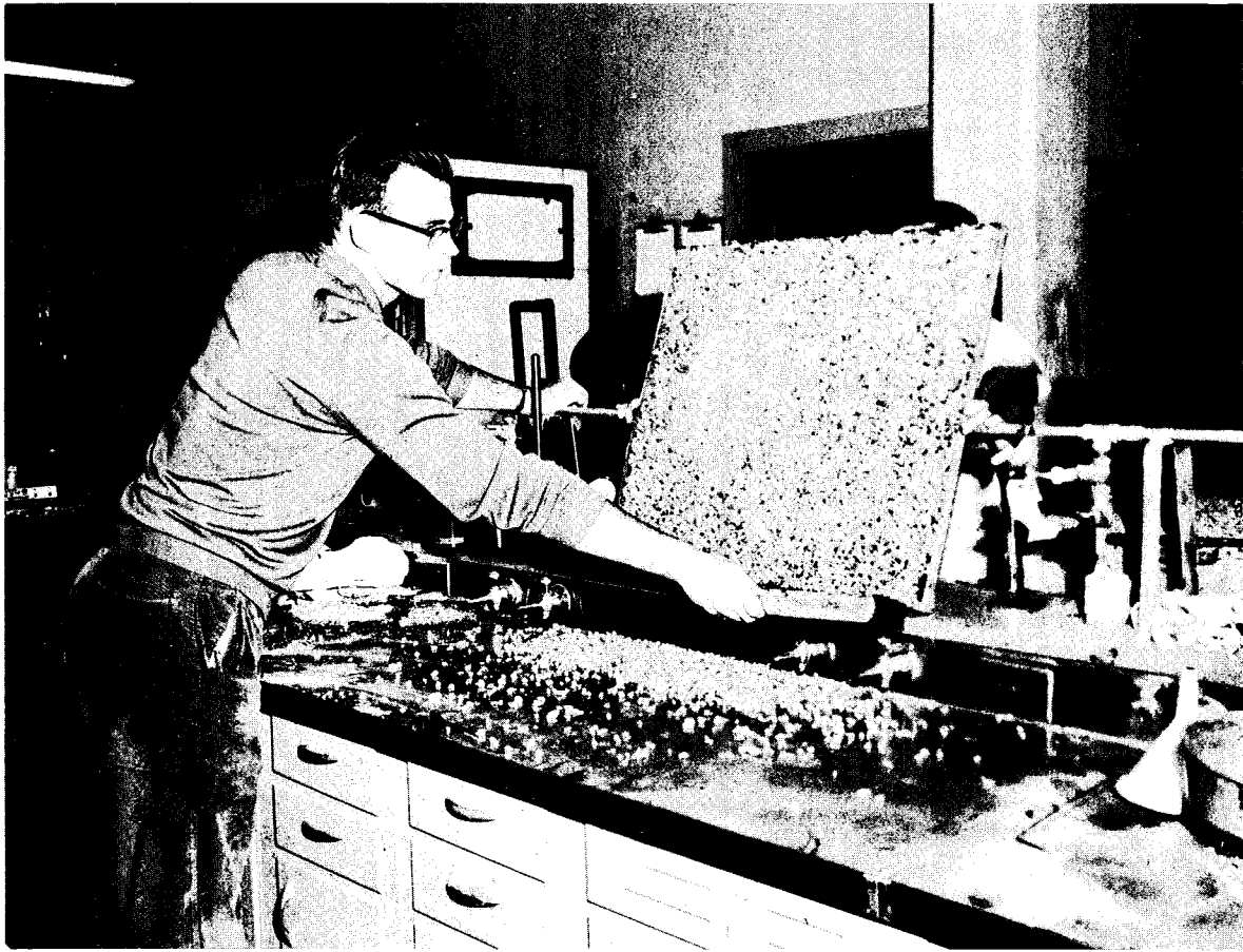
Figure 16. Completed surface is tilted at 75^{\circ} and brushed to remove loose stone.
