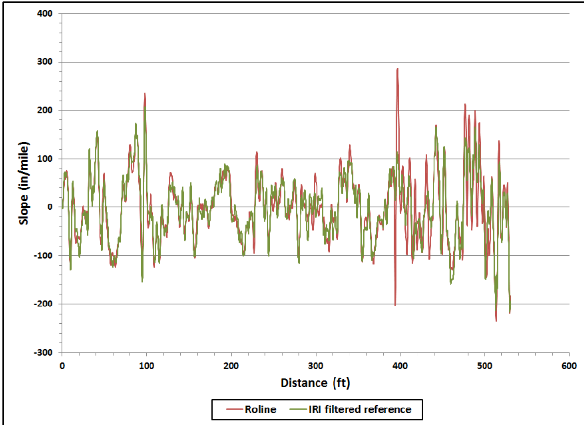
Figure 58. Comparison of IRI Filtered Profiles on a Section of CRCP Test Track.
