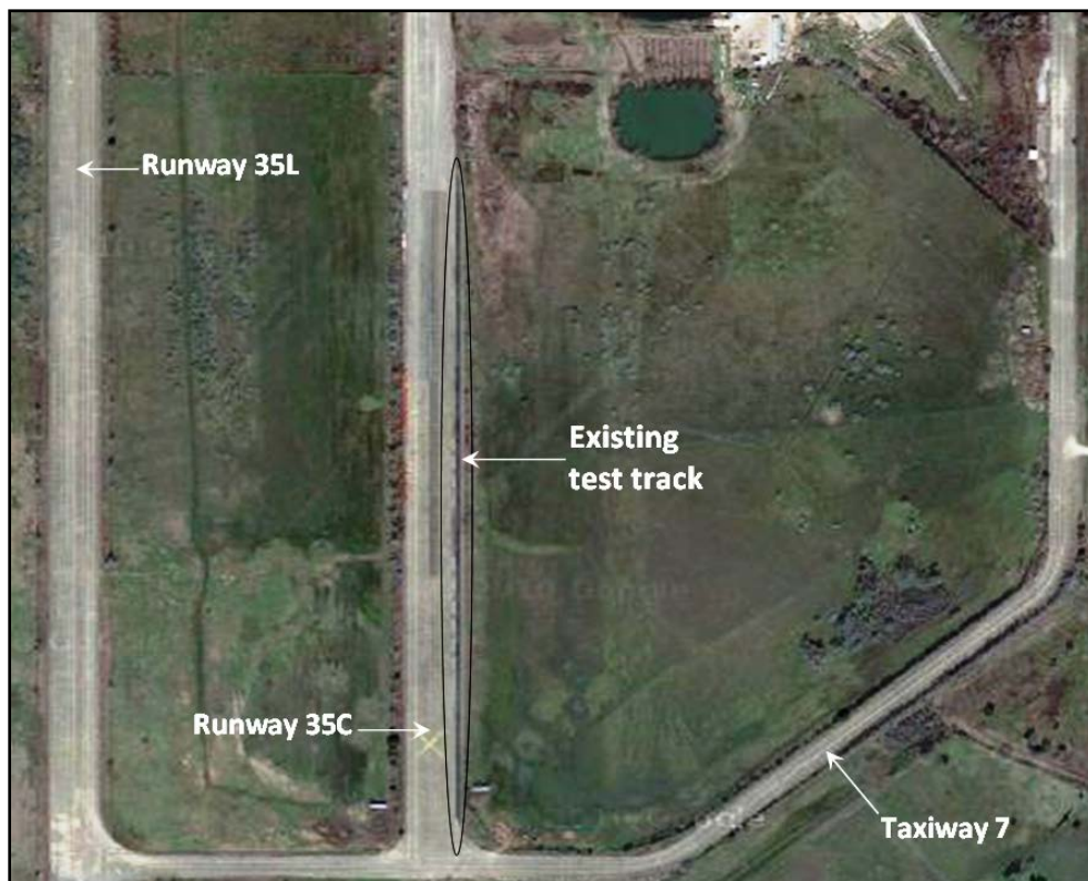
Figure 1. Existing Test Track Used for Inertial Profiler Certifications.
