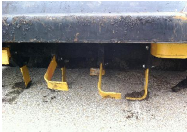
Figure 12. Milling and Scarifying Teeth.
