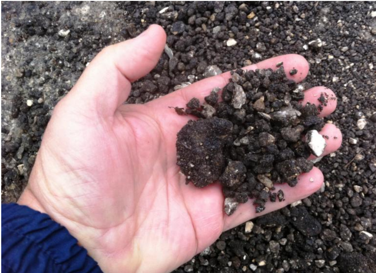
Figure 15. Size Distribution after First Milling Pass.
