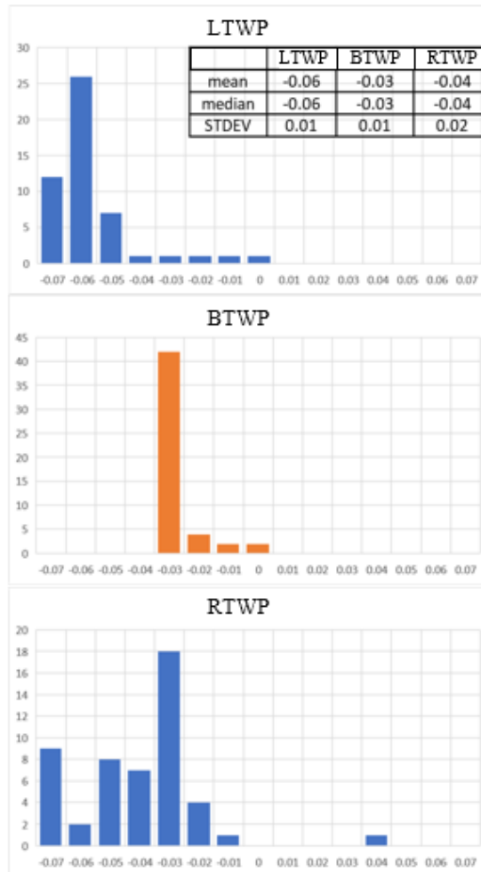
Figure 9. Distribution of Binder Rate Adjustment Output for 1 Mile of FM 2095 EB (horizontal axis: rate adjustment; vertical axis: distance ft).
