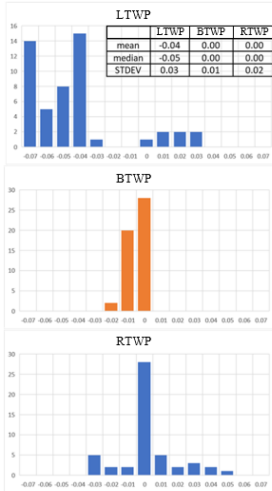
Figure 10. Distributions of Binder Rate Adjustment Output for 1 Mile of FM 1915 NB (horizontal axis: rate adjustment; vertical axis: distance ft).
