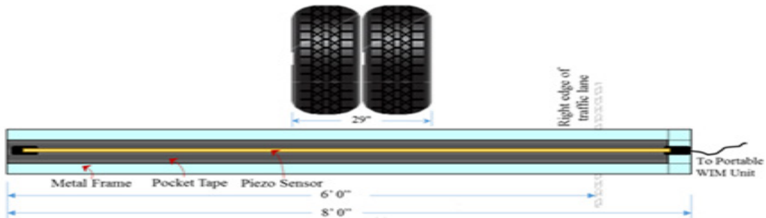
Figure I-3. Schematic View of the Metal-Plate and Sensor Setup.
