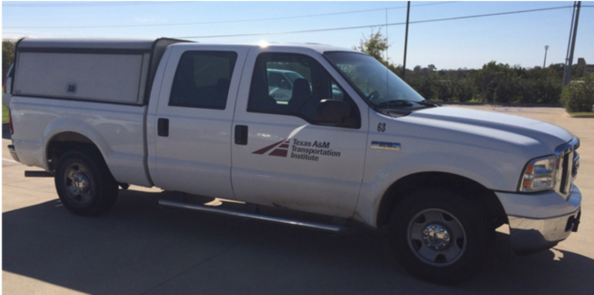
Figure IV-3. TTI Class 03 Truck for Portable WIM Calibration
