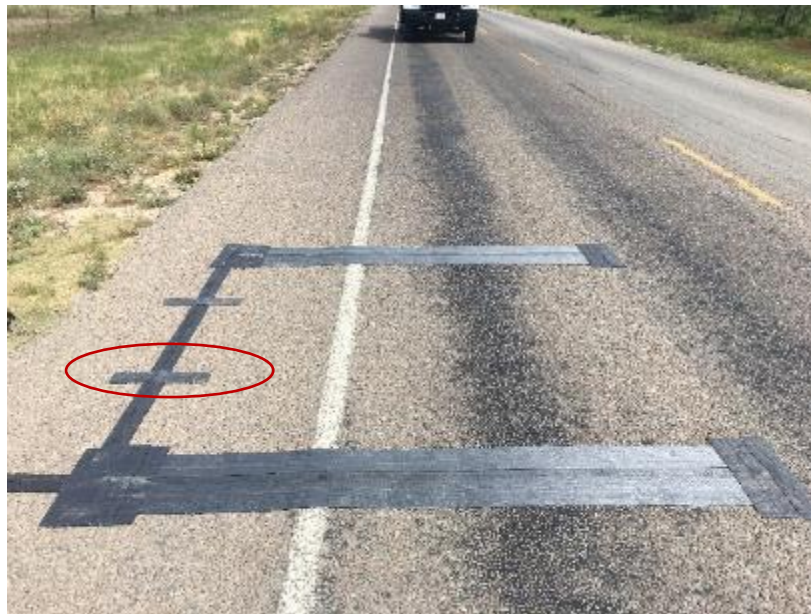
Figure 43. Horizontal Road Tapes (about 20-Inch Long).
