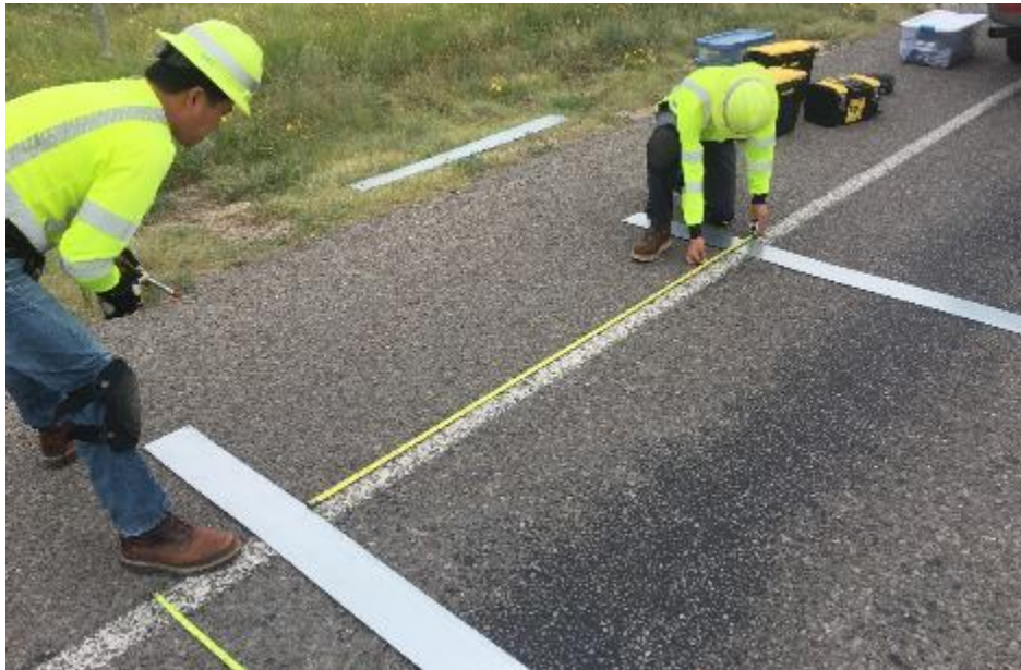
Figure 31. Measuring Distance between Each Metal Plate.
