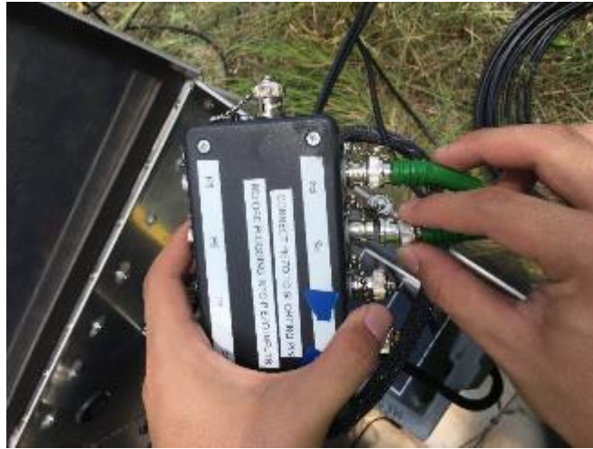
Figure 46. Connecting the Sensor Cables to the Piezo Channel Box.
