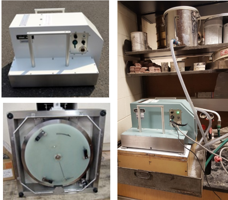
Figure 3. DFT Test; (a) Apparatus Side View (2), (b) Apparatus bottom View (2), and (c) TxDOT Setup.
