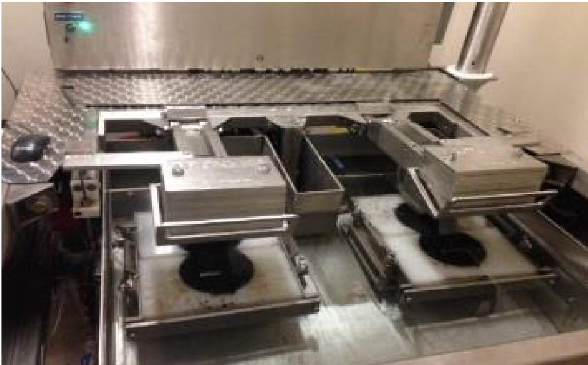
Figure 5. Typical HWTT Test Setup.
