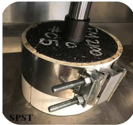
Figure D-4. SPST Specimen Setup.
