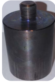
Figure D-1. Loading Head.
