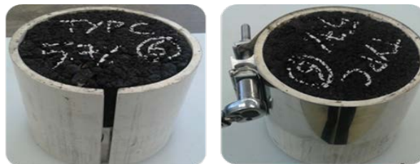
Figure 3. SPST sample confinement: Cylindrical enclosure and collar strap.
