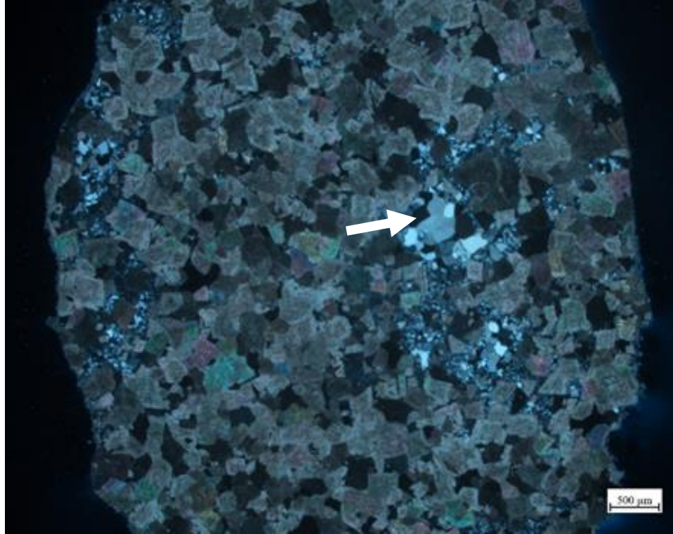
Figure 16. Siliceous Inclusions (White) within a Limestone Particle.
