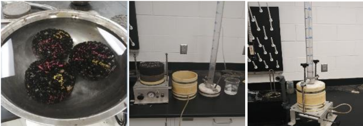
Figure 13. Permeability Test Using the Florida Test Method.
