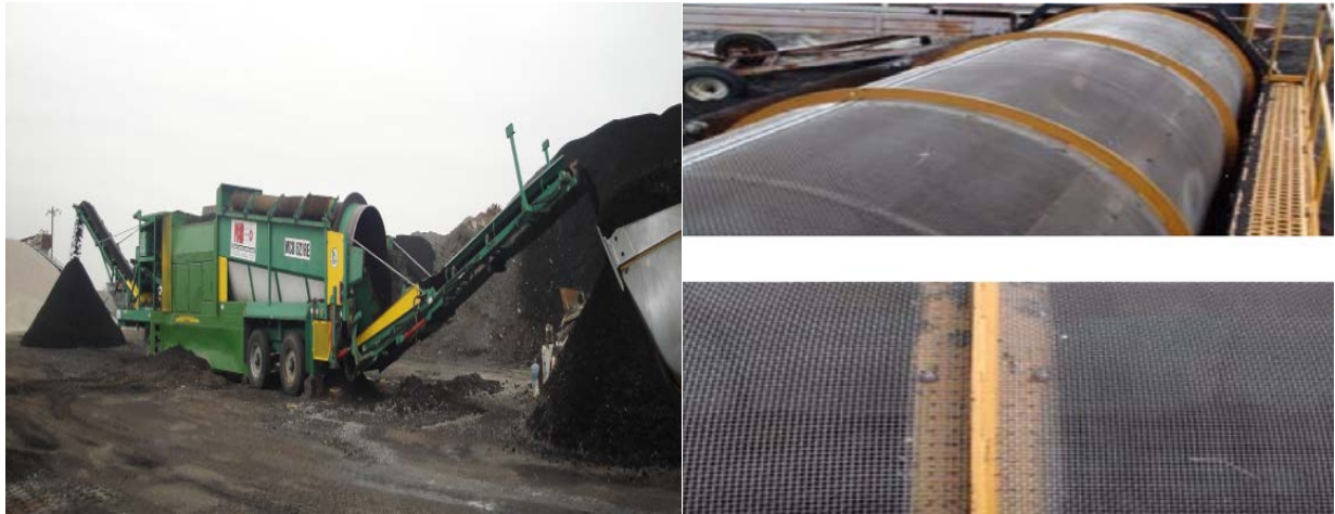
Figure 6. Screening RAS Using Trommel Screen Machine.
