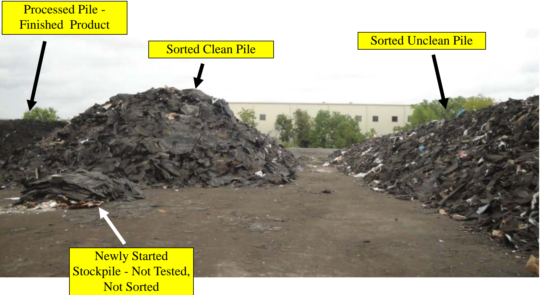
Processing RAS - Sort Piles
