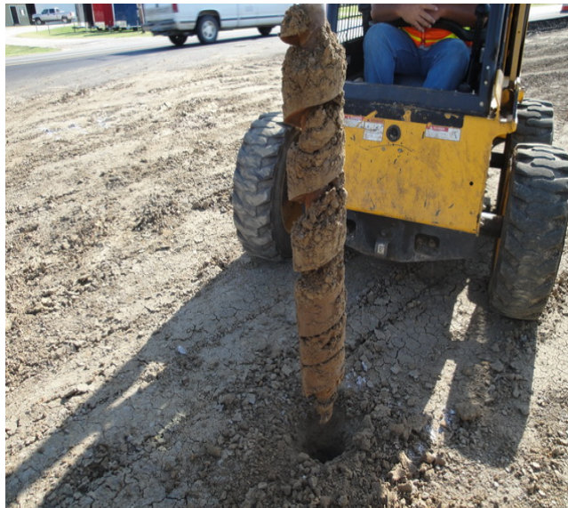
Figure 3-3. Auger Used to Collect Soil Samples (Every 1 Ft to a Depth of 4 Ft).
