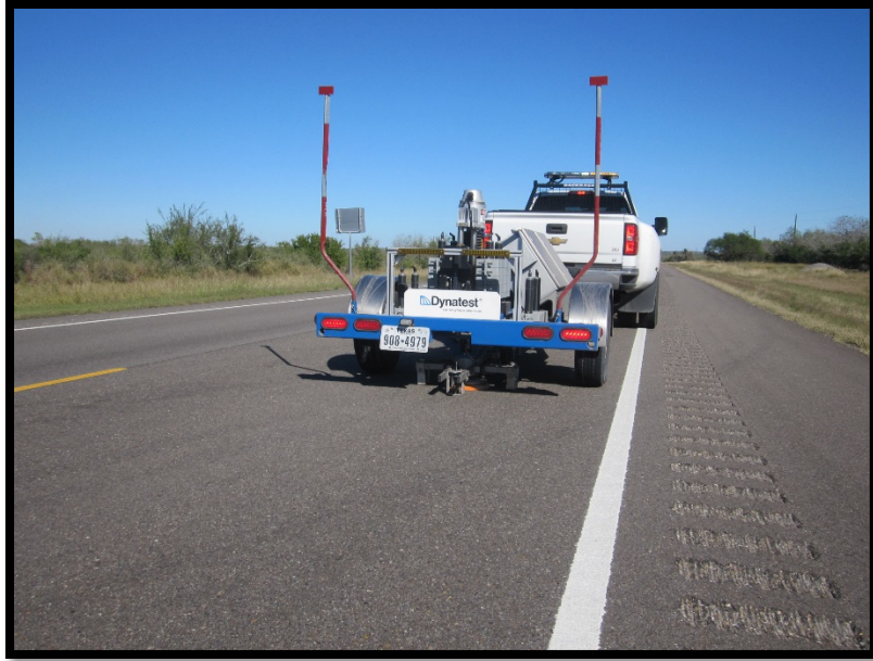
Figure 15. FWD Collection on Completed US 59 Mill and Inlay.
