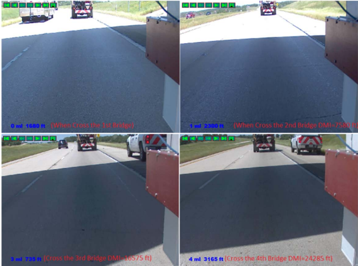
Figure 40. Video Frames Showing the TPAD Going under the Bridge.
