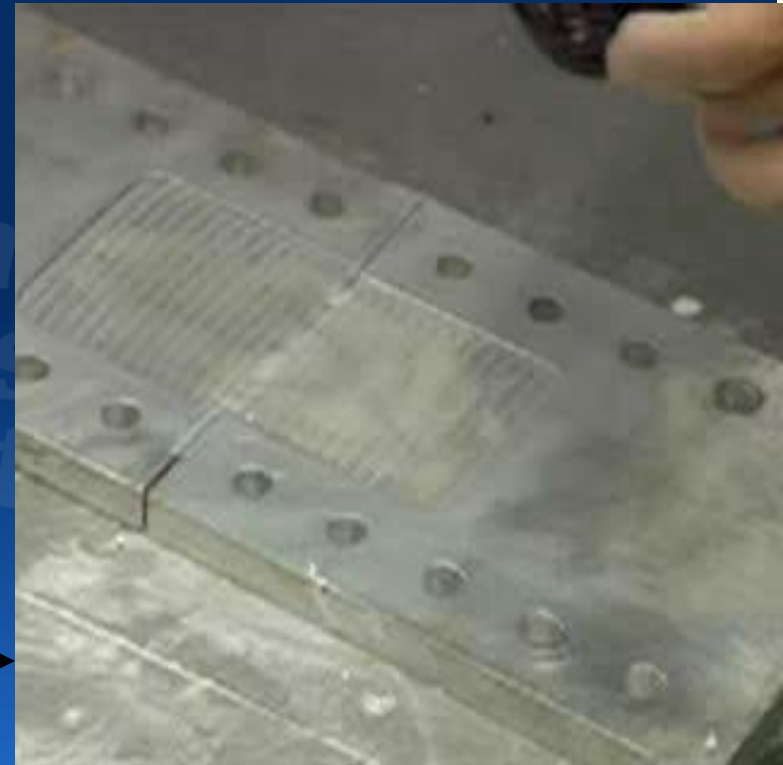
Reflection Cracking test
