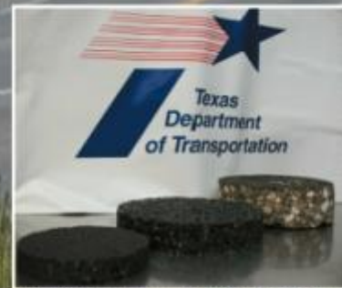
TXDOT's longer-lasting, thinner 1-inch and half-inch overlay alternatives use finer aggregates than the traditional 2-inch overlay, resulting in safer, smoother rides for motorists.
