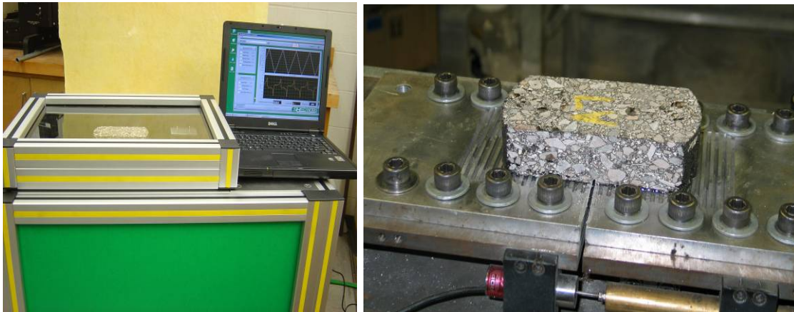
Figure 2. Overlay Tester Equipment and Sample.
