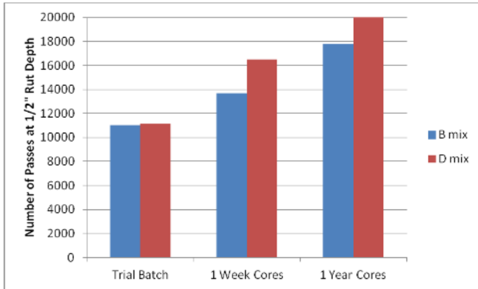
Figure 3.20. Hamburg Wheel Tracking Test Results for Type B and Type D WMA on BU 287.
