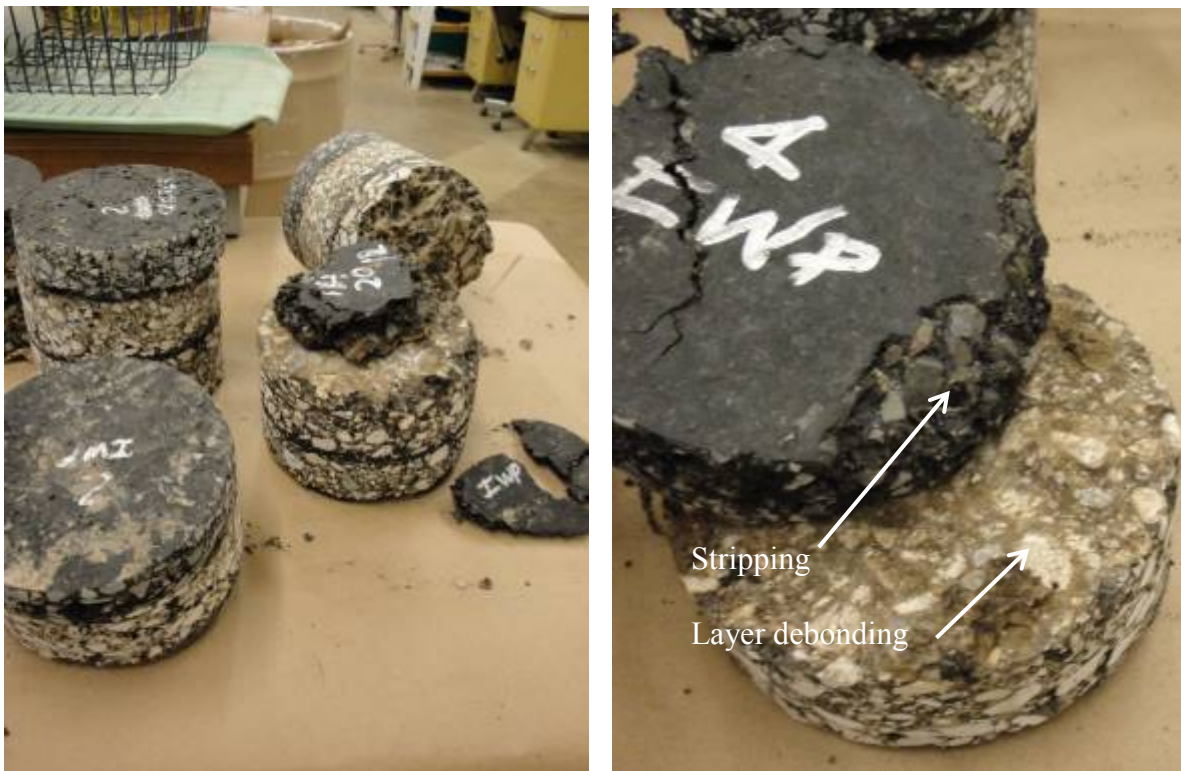
Figure 3.41. Flushed and Moisture Damaged Core Specimens (Atlanta-Fine SMA).
