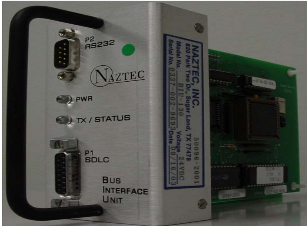
Figure 2. TS-2 Cabinet Enhanced BIU.
