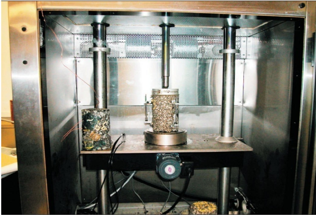
Figure 4-1. Dynamic Modulus Test Equipment and Specimen.
