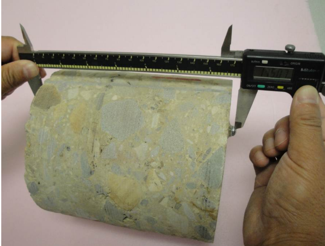
Figure 6-13. CTE Measuring of CTB Material.
