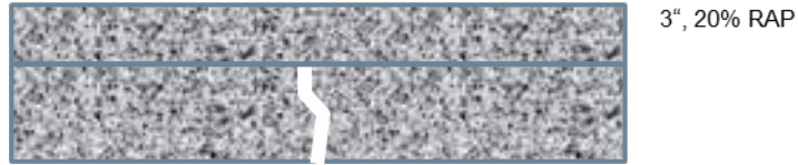
Figure 3-26. Schematic Diagram of SH 359 Pavement Structure.
