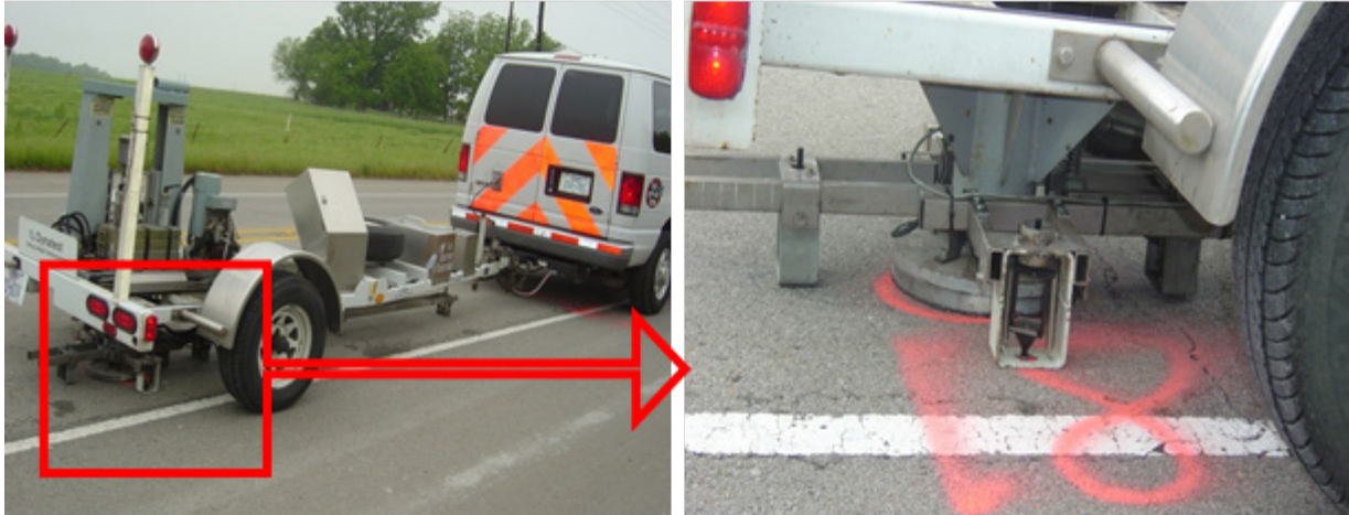
Figure 4-15. FWD Test with the Loading Plate at One Side of Crack.
