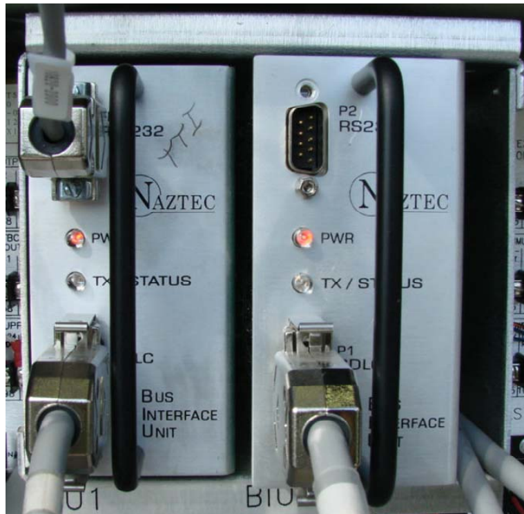
Figure 15. Enhanced BIU with a Serial Port.
